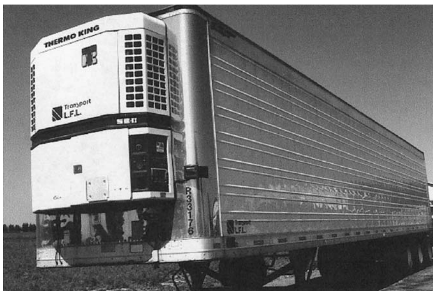
Fig. 3 Nose-mounted refrigeration system used in a semitrailer.
