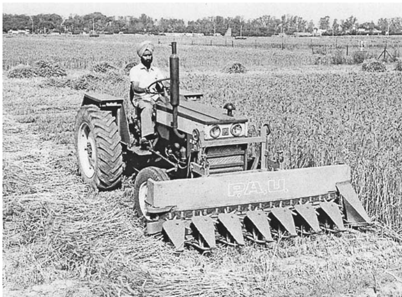
Fig. 16 Tractor front-mounted vertical conveyor-reaper-windrower: observe the crop windrow. (Courtesy of Punjab Agricultural University, Ludhiana, India.)
