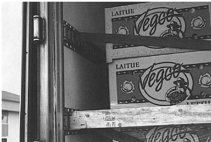
Fig. 1 Bracing system using straps and wooden bars to hold produce boxes.
