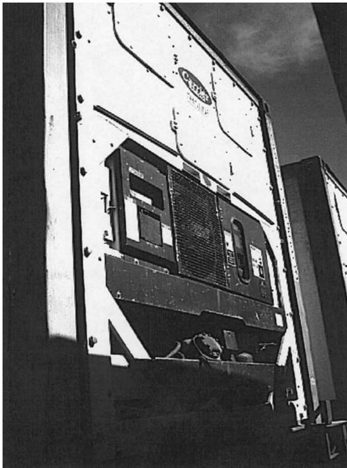
Fig. 4 Recessed refrigeration system fused with the front wall of an intermodal container.
