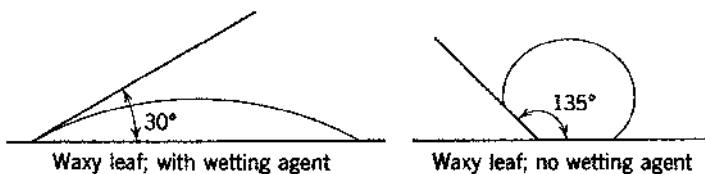
Figure 7-3. Left: Water droplets containing a wetting agent will spread in a thin layer over a waxed surface. Right: Pure water will stand as a droplet, with only a small area containing the surface wax.
