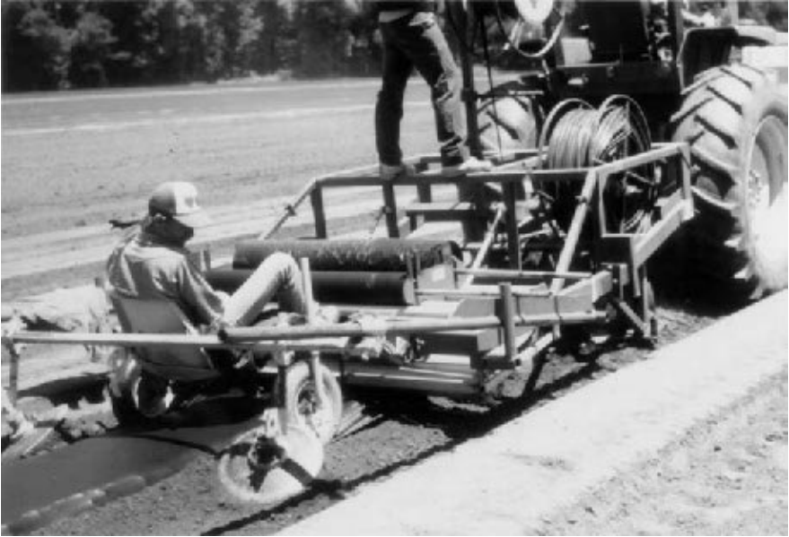
Figure 17-1. Methyl bromide fumigation applicator that injects the fumigant into the soil and then places a sealed plastic tarp over the treated soil to contain the gas in the soil atmosphere. (D. Sanders, North Carolina State University.)
