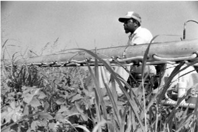
Figure 7-12. Rope-wick applicator. Herbicide-soaked ropes are attached to a horizontally positioned pipe reservoir. (Southern Weed Science Laboratory, USDA-ARS, Stoneville, MS.)
