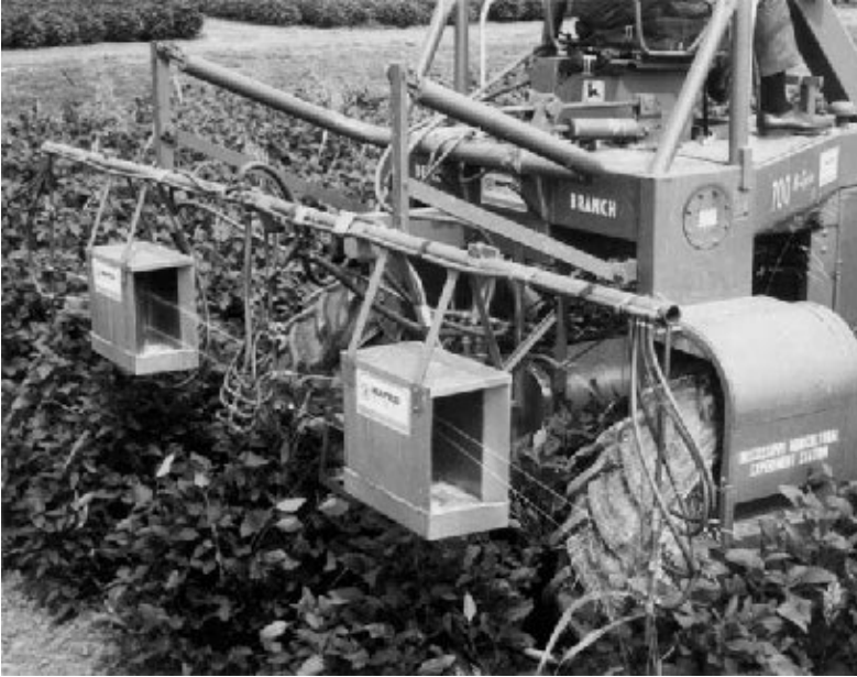
Figure 7-11. Recirculating sprayer equipped with solid-stream nozzles to apply herbicides to weeds that are taller than the crop. Spray caught in the box is returned to the tank to be sprayed again. (Southern Weed Science Laboratory, USDA-ARS, Stoneville, MS.)
