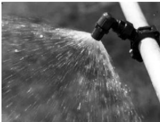
Figure 7-9. Raindrop (brand) nozzle spraying at 40 psi. (Photo by Ann Hawthorne, Delavan Corporation.)
