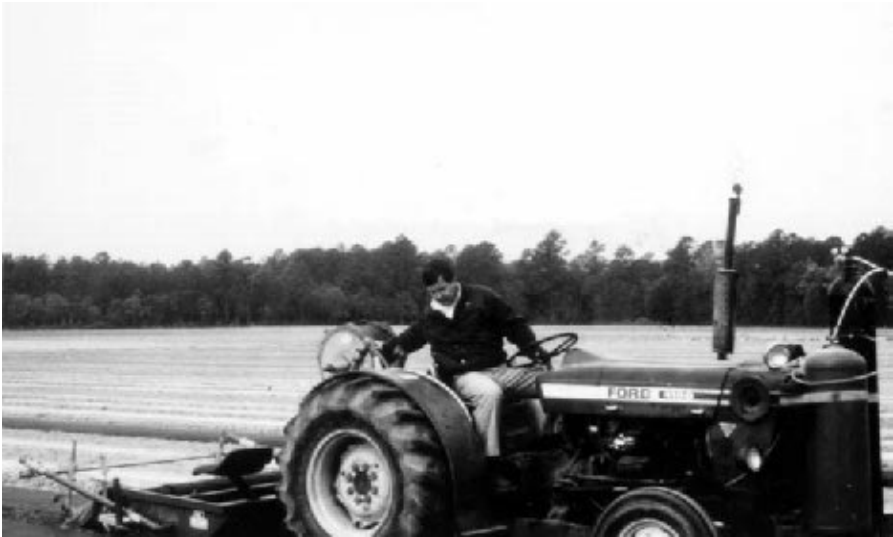
Figure 23-4. Methyl bromide fumigation equipment. The methyl bromide is injected into the soil on the plant beds and immediately covered with a plastic tarp. (D. Sanders, North Carolina State University.)
