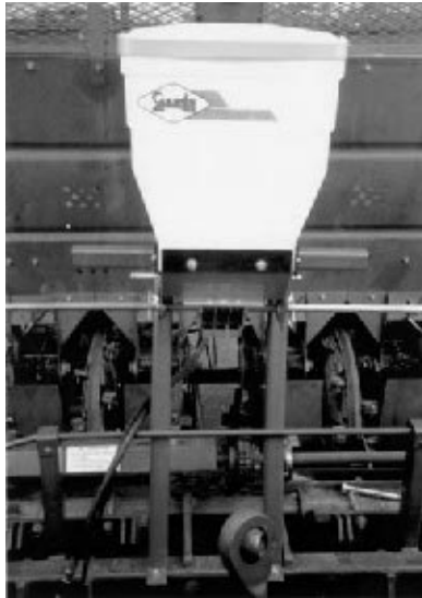
Figure 7-13. Applicator for banding granular materials over plant rows at planting time. (Gandy Company.)
