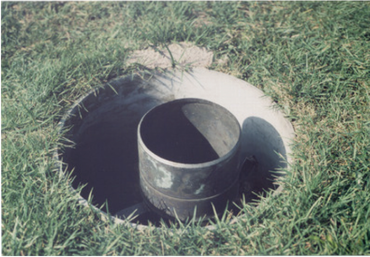
Fig. 3.1 The equipment used to measure precipitation influences the quantity measured where, the catch diameter, elevation, and surrounding ground cover all influence accuracy
