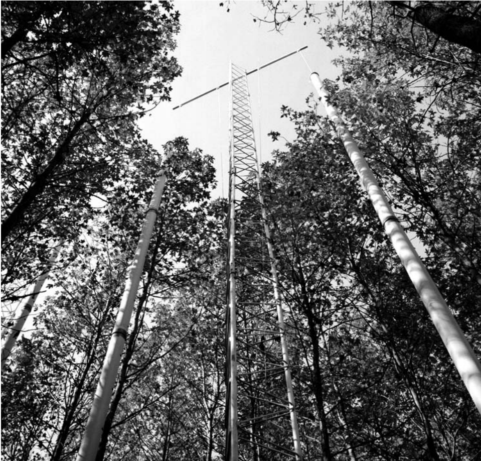
Figure 8.3. The Tennessee FACE site showing the towers used to release \text{CO}_2 into the forest. Source: Rich Norby/ORNL FACE.
