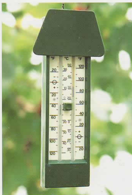
Above: A maximum/minimum thermometer is an essential tool in helping you to judge the conditions in your greenhouse.
