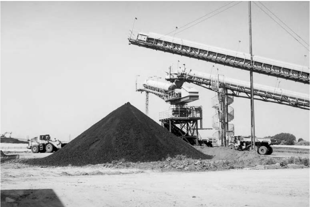
Sorting and treatment of sediment dredged from the River Elbe, Hamburg, Germany (photo: P.N. Owens).
