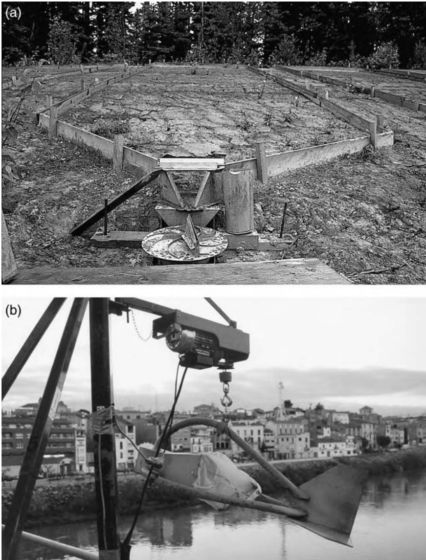
Fig. 28.1. (a) Erosion plot and Coshocton-wheel, Stuart-Takla Research Forest, British Columbia, Canada (photo: E.L. Petticrew); and (b) Helley-Smith bedload sampler, Ebro River, Spain (photo: P.N. Owens).
