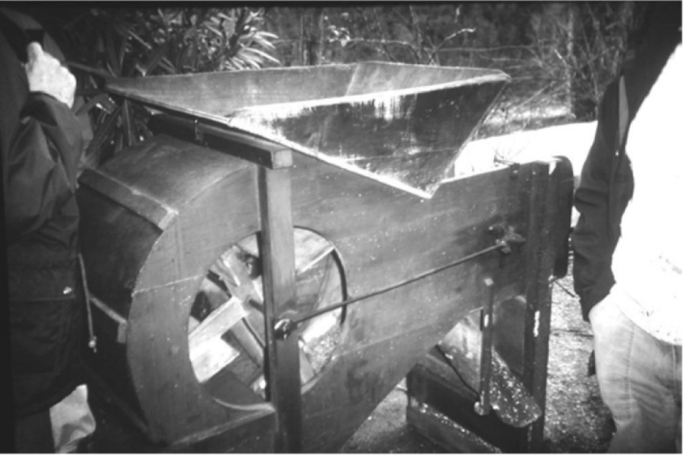
Figure 25. Traditional machine to spare chestnuts from burs.
