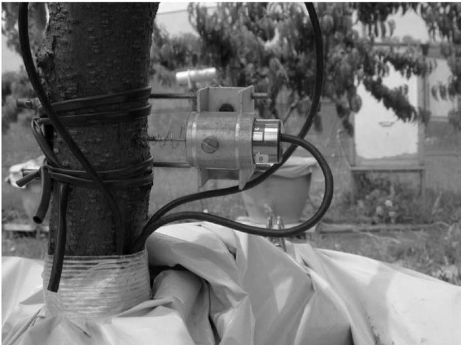
Plate 1. Trunk shrinkage is measured using a linear variable differential transformer (LVDT) mounted on an INVAR frame.
