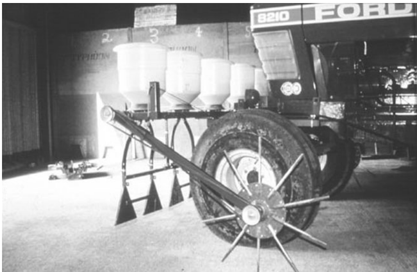
Fig. 16.2. Horstine Farmery Microband Applicator showing hoppers and 'fishtail' distribution units.
