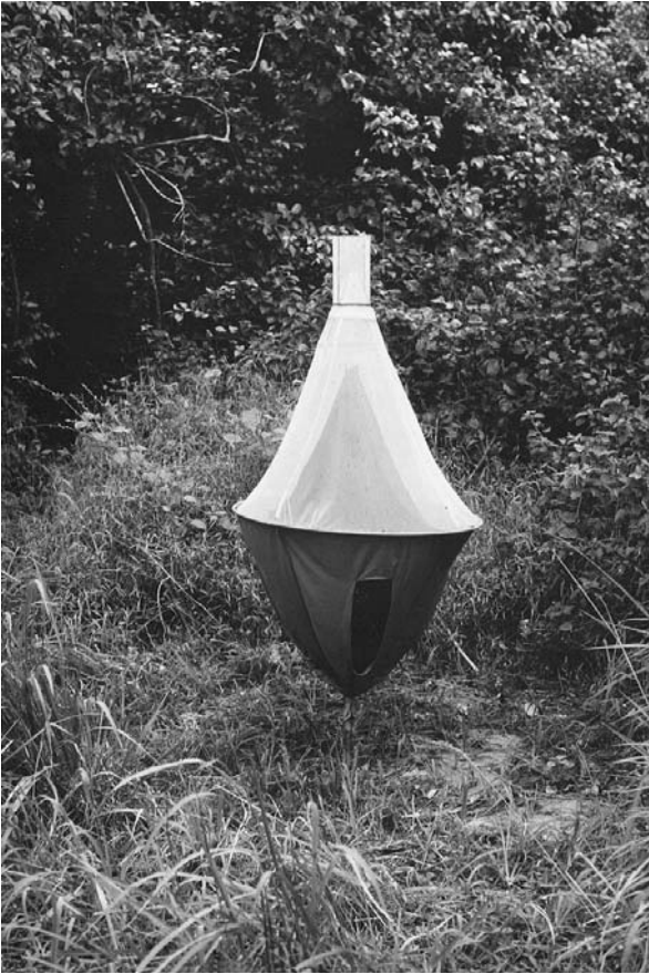
Fig. 12.7. A biconical trap used to 'trap out' tsetse populations and so control African trypanosomiasis (M. W. Service).
