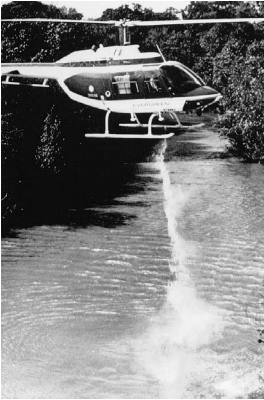
Fig. 4.15. Helicopter dropping temephos insecticide into a stream to kill larvae of simuliid black flies (Courtesy of J. B. Davies).
