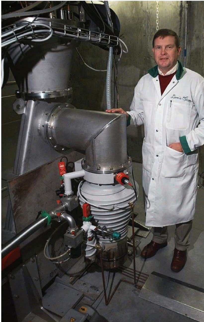
Dennis Olson, director of irradiation research at Iowa State, stands next to the linear accelerator used to zap meat with radiation. Opponents of irradiation believe that the process could be harmful to humans.
