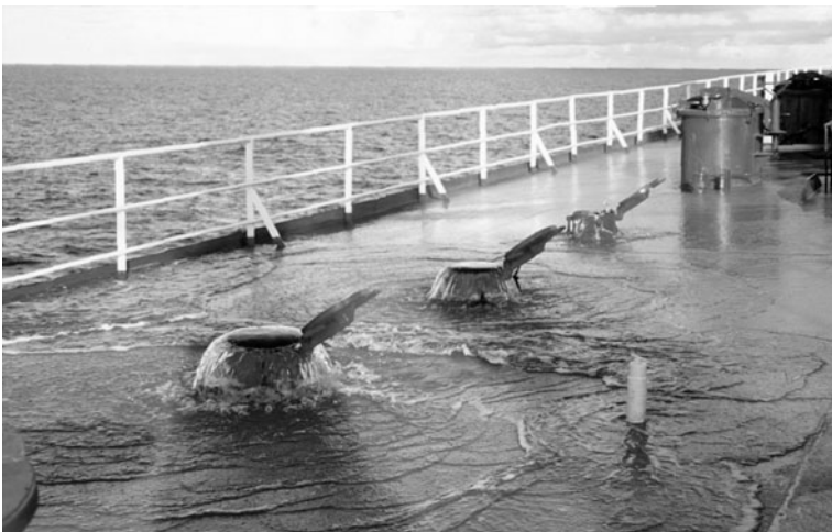
Fig. 14.2 Ballast water overflowing from inspection ports on a tanker vessel undertaking mid-ocean ballast water exchange. Photo: T. Dodgshun, Cawthron Institute.
