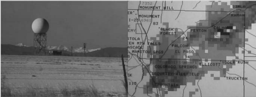
Fig. 2.4 National Weather Service WSR-88D Doppler radar at Pueblo County, Colorado, USA and example of Storm Total Precipitation output ( http://www.crh.noaa.gov/pub/?n=/radar_about.php )
