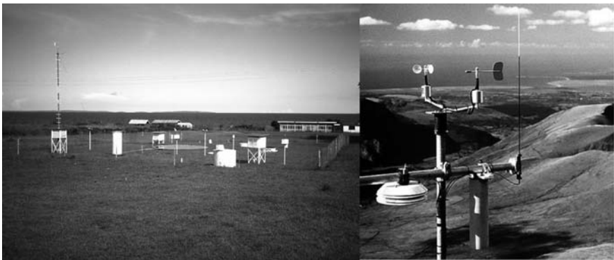
Fig. 2.3 Example of (a) a manually operated weather station and (b) an automatic weather station installed at the top of Mount Snowdon in Wales, including an antenna for radio telemetry of data (© Crown Copyright 2008, the Met Office)
