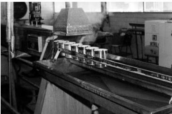
Figure 5 Vapor tunnel or exhauster.
