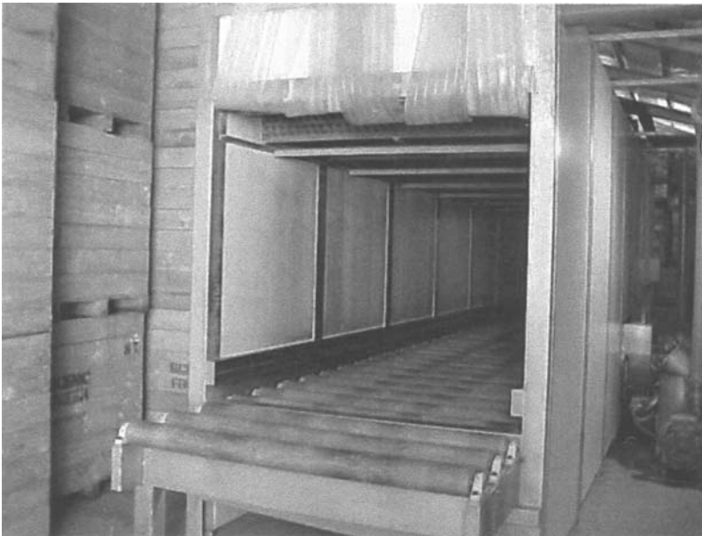
Figure 10 Hydrocooler used for cooling of harvested vegetables. (Photo courtesy of GROPAK, Palmerston North, NZ.)
