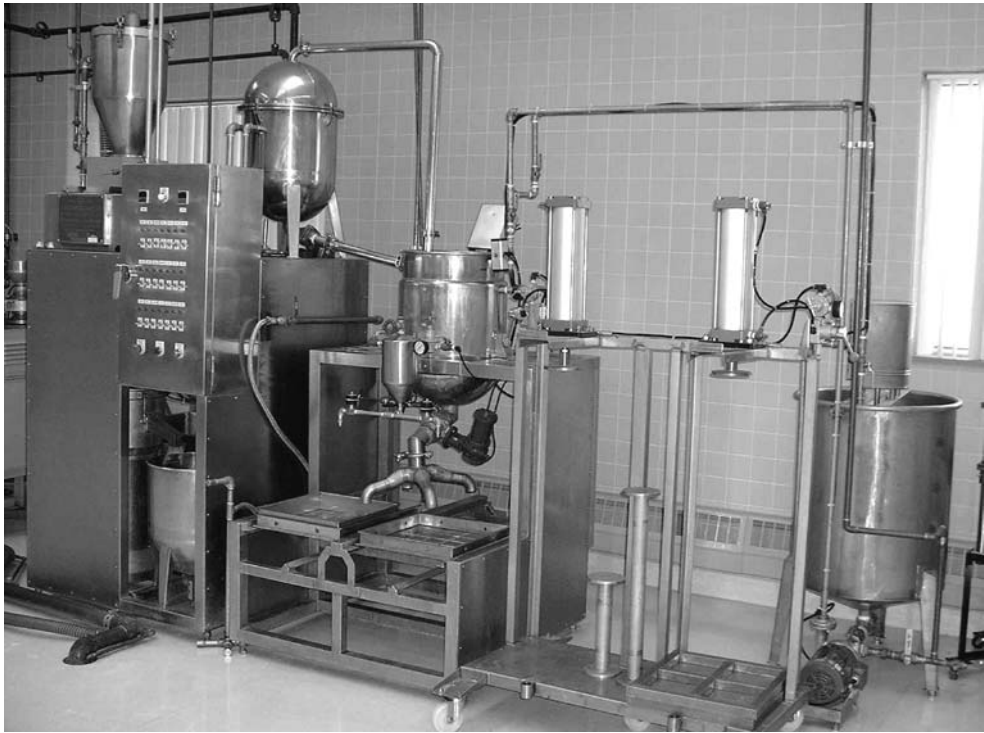
Figure 13 The automatic production-scale machine (made by Ta-Ti-Hsing Machinery Co., Taoyuan, Taiwan) for soymilk and tofu production at North Dakota State University.
