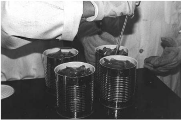
Figure 4 Three-sheet tin cans covered inside with porcelain enamel.
