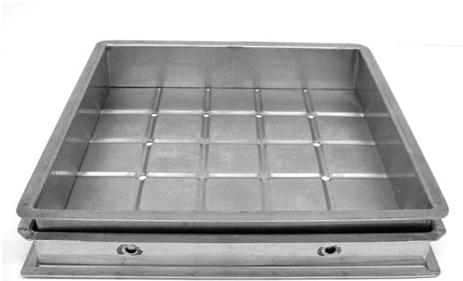
Figure 12 The tofu mold used by the production-scale machine at North Dakota State University. (Size: 40L × 40W × 4.5Hcm.)
