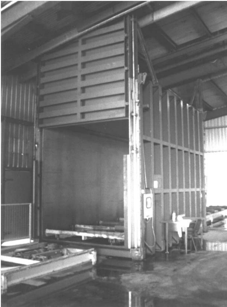
Figure 11 Vacuum cooler used for cooling of harvested vegetables. (Photo courtesy of Intercoast Express Pty. Ltd., Werribee South, Victoria, Australia.)
