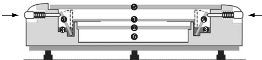
FIGURE 9.4 Horizontal developing chamber (Camag): 1, chromatographic plate with layer face down; 2, counter plate (removable); 3, troughs for solution of the mobile phase; 4, glass strip for transfer of the mobile phase by capillary action to the chromatographic plate; 5, cover glass plate. (Courtesy of Camag, Muttenz, Switzerland, www.camag.com )
