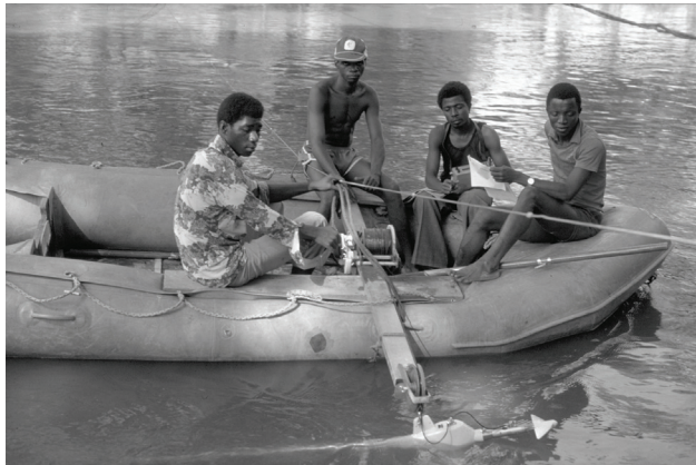
Fig. 8.18 : Gauging with a current meter from a boat.
