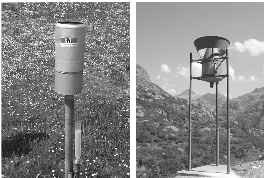
Fig. 8.1 : Plain and mountain installations of accumulative rain gauges.
