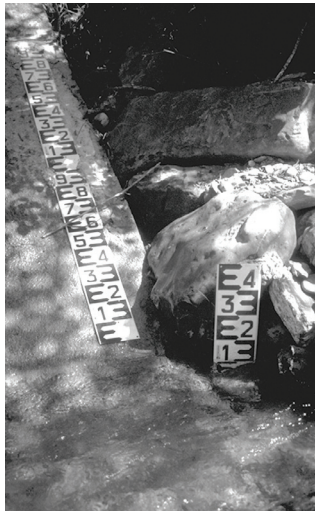
Fig. 8.12 : Inclined and vertical staff gauges.
