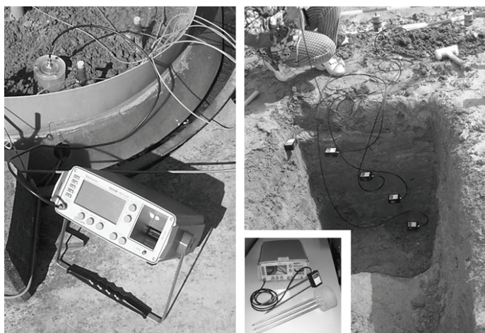
Fig. 8.30 : TDR probe and different types of electrodes in the soil.
