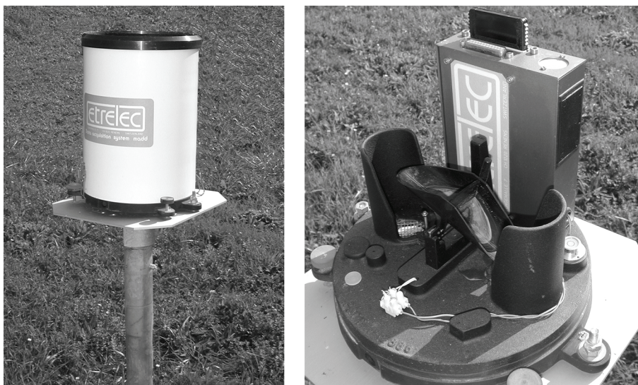
Fig. 8.4 : Tipping-bucket rain gauge and MADD recording system.
