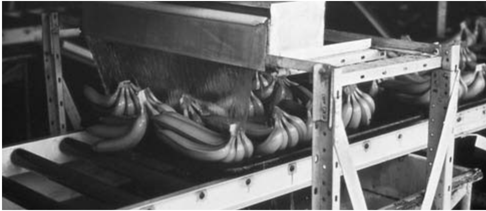
Figure 12.32 A cascade fungicide applicator in a in a packhouse in Ecuador.
