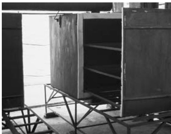
Figure 12.70 Chamber for on farm fumigation of litchis with sulphur dioxide in Thailand.
