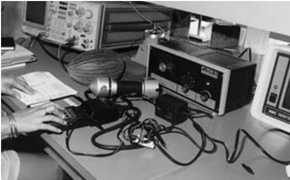
Figure 2.5 A colour difference meter being used to measure the colour of melons. Source: Mr A.J. Hilton.
