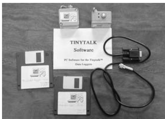
Figure 11.10 A small temperature logger that can be used to monitor the condition inside boxes of fruit and vegetables during transport. Source: Dr J.R. Robinson.
