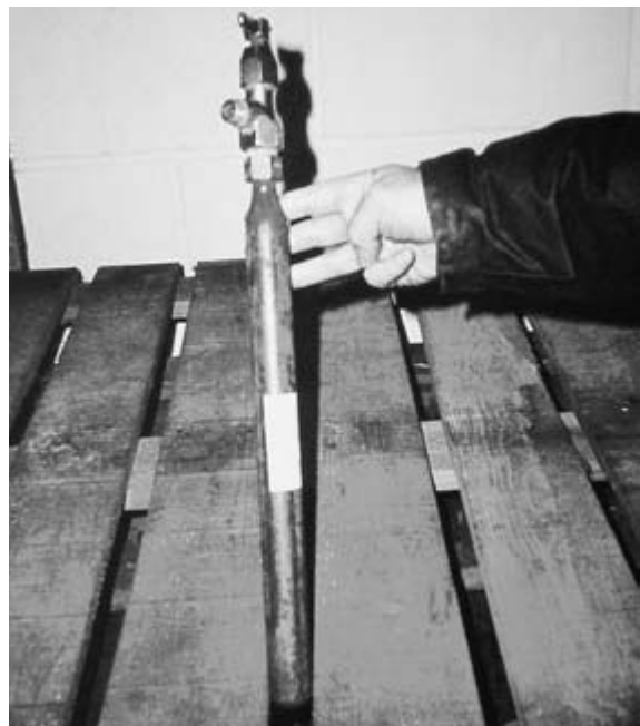
Figure 10.5 Small cylinders of ethylene called lecture tubes used for ripening of fruit.
