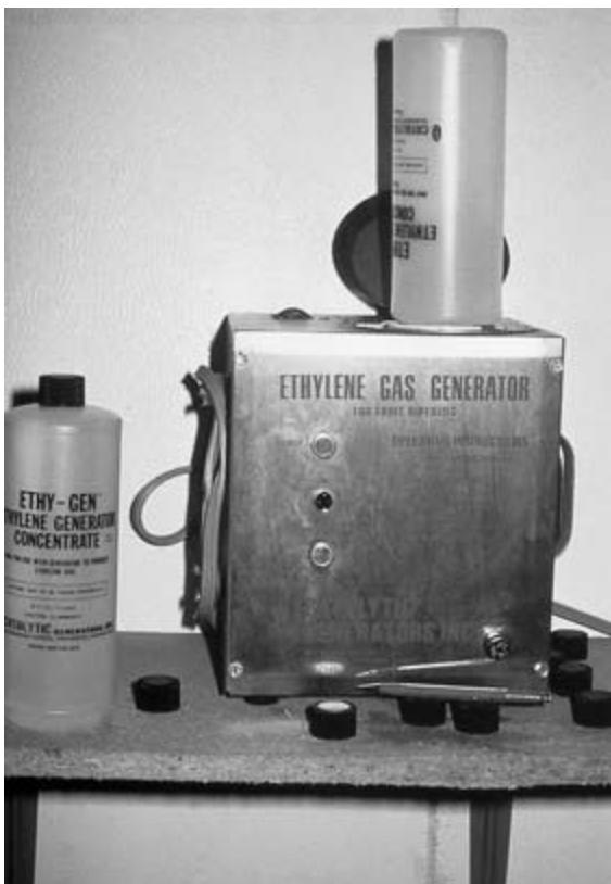
Figure 10.6 Commercially available ethylene generator of the type commonly used to initiate fruit ripening showing the bottles of liquid which are poured into the generator.
