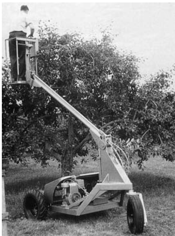
Figure 3.3 A platform used to facilitate fruit harvesting from tall trees in the UK.
