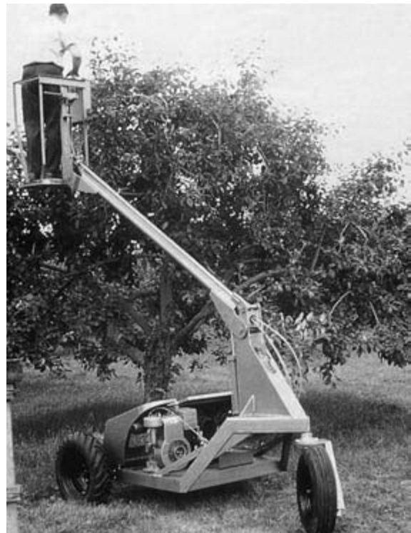
Figure 12.4 A platform used to facilitate fruit harvesting from tall trees in the UK.
