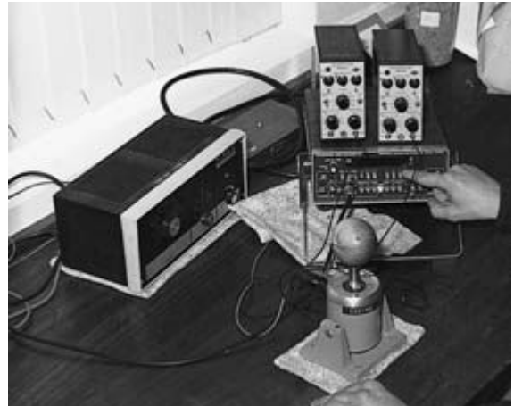
Figure 2.6 Equipment which puts vibrational energy into fruit and measures its response being tested on apples. Source: Mr A.J. Hilton.
