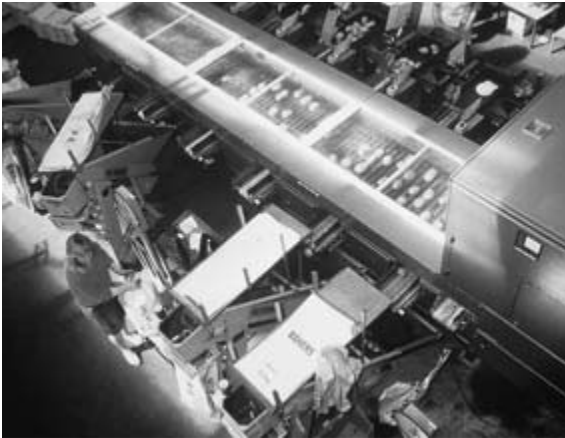
Figure 2.1 An on-line colour sorting machine being used on potatoes.
