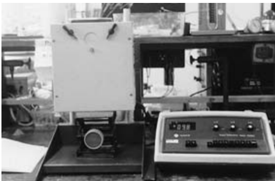
Figure 2.4 Experimental equipment used for testing changes in diffuse light in fruit. Source: Mr A.J. Hilton.
