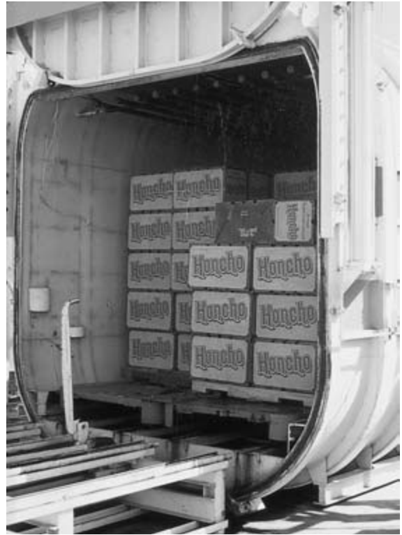
Figure 4.5 The inside of a vacuum cooler with water spray facilities used for precooling lettuce in California where it is called 'Hydrovac'.
