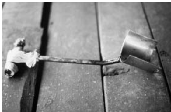
Figure 12.28 A chisel type of dehanding tool being used in a packhouse in Ecuador.
