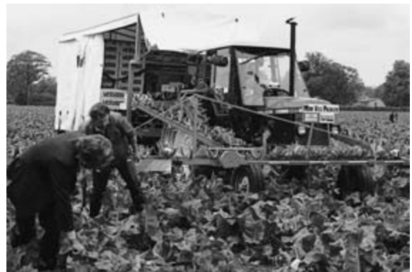
Figure 3.4 Tractor-mounted conveyer belt to facilitate hand harvesting with a trailer used for field packing.
