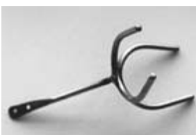
Figure 12.20 Metal banana callipers with the maximum acceptable finger diameter at one end and the minimum at the other. These are fixed to a pole so that the diameter can be measured from the ground.
