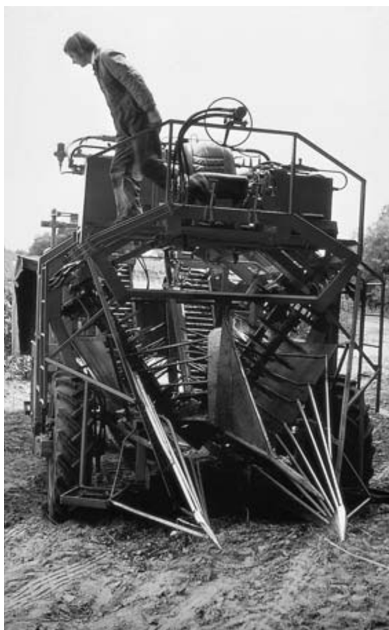
Figure 12.40 Mechanical harvester used for blackcurrants for processing into juice in the UK. Source: Professor H.D. Tindall.
