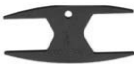
Figure 12.19 Plastic banana callipers with the maximum acceptable finger diameter at one end and the minimum at the other.
