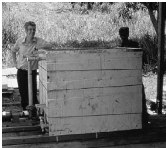
Figure 12.75 A batch mango hot water treatment facility erected on a farm in St James, Jamaica.
