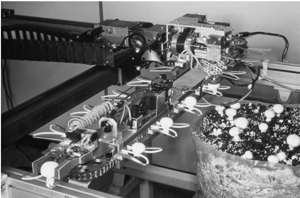
Figure 12.78 Robotic mushroom harvester developed at the Silsoe Research Institute. Source: Dr Robin Tillet.
