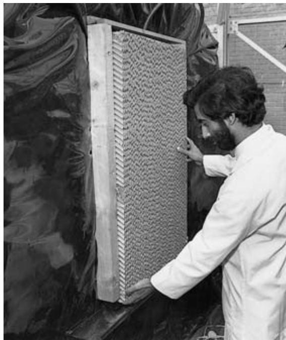
Figure 7.10 An experimental evaporatively cooled store showing the constantly moistened Celdec pad through which the air is passed to cool the insulated store. Source: Mr A.J. Hilton.
