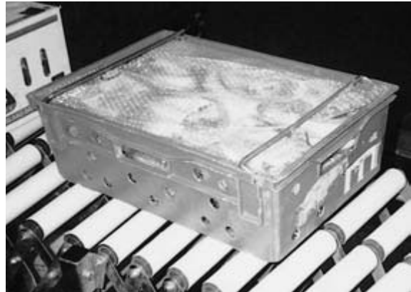
Figure 12.35 Reusable collapsible plastic box from the IFCO design used in banana transport trials from the Windward Islands to Britain.
