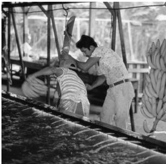
Figure 12.27 Fruit being dehanded and placed in a delatexing tank in a packhouse in Ecuador.
