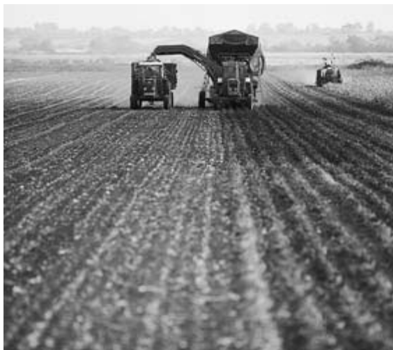
Figure 12.81 Onion harvesting where the leaves have been cut off and the harvesting machine is lifting them and transferring them directly to a tractor and trailer alongside.
