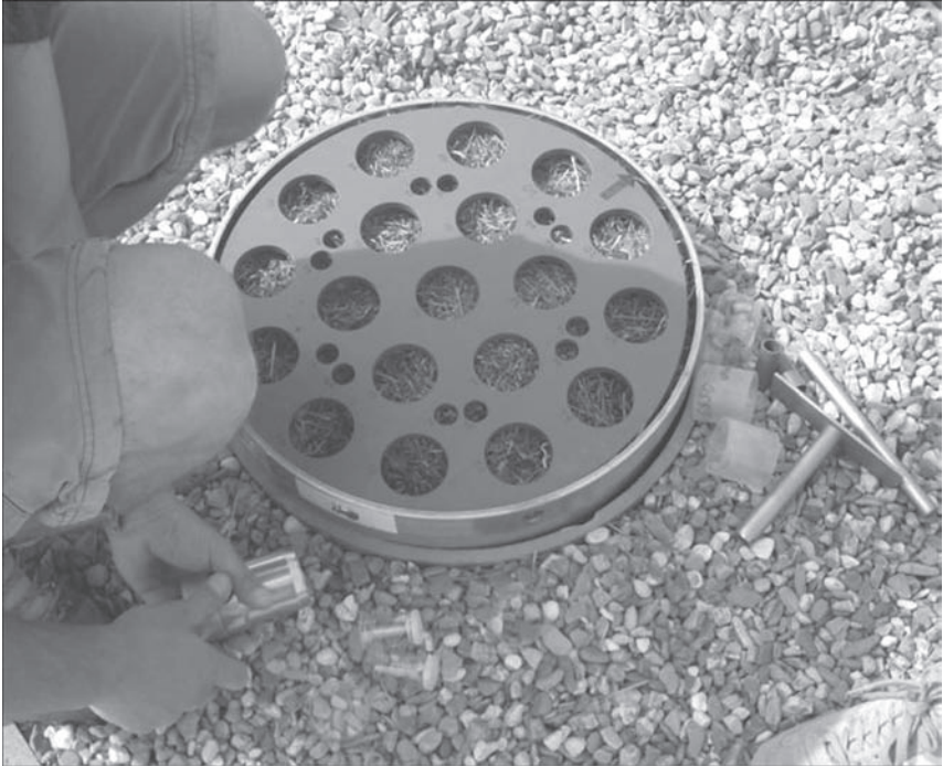
FIGURE 4.6 The surface area of a TME (diameter 47 cm) allows for sequential coring of up to 19 subsamples for extracting enchytraeids or microarthropods and several small cores. (Photo by Bernhard Theißen.)
