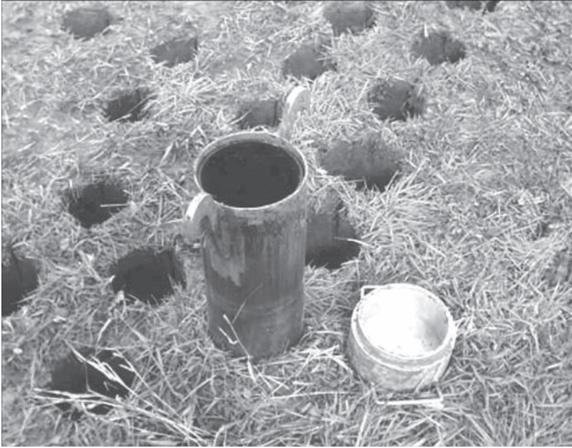
FIGURE 5.2 Extraction of TME soil cores from a central European meadow site. (Photo by Bernhard Förster.)
