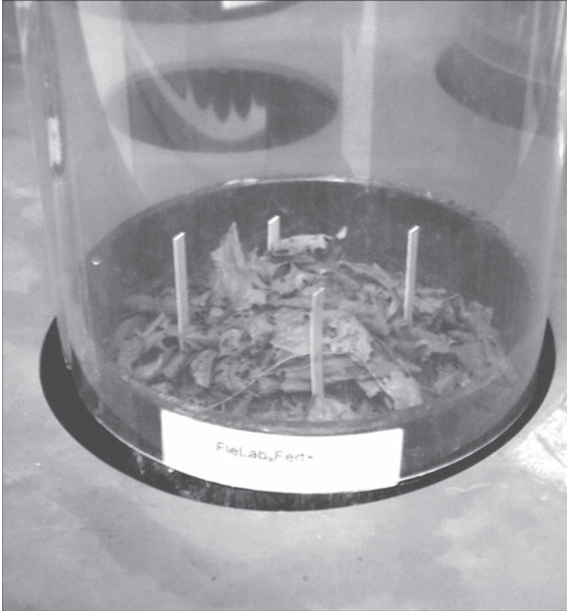
FIGURE 5.3 Conducting a bait-lamina test in a TME extracted from an agroforestry site. (Photo by Bernhard Förster.)
