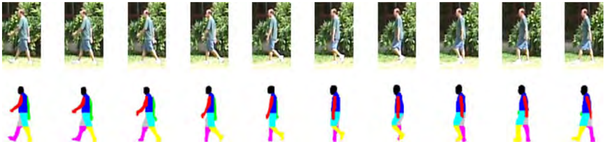
Evaluation of Gait Recognition. Figure 4 Top row shows the color images, cropped around the person, for one sequence. The bottom row shows the corresponding part-level, manually specified silhouettes.
