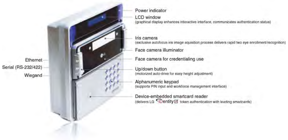
Iris Acquisition Device. Figure 5 An example of the IrisAccess 4000 (from http://www.lgiris.com/ps/products/irisaccess4000.htm ).
