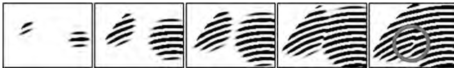
Fingerprint Sample Synthesis. Figure 10 Genesis of a minutia point during the merging of the two regions originated by two different initial points.
