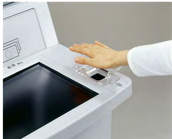
Palm Vein. Figure 5 ATM with palm vein authentication sensor.
