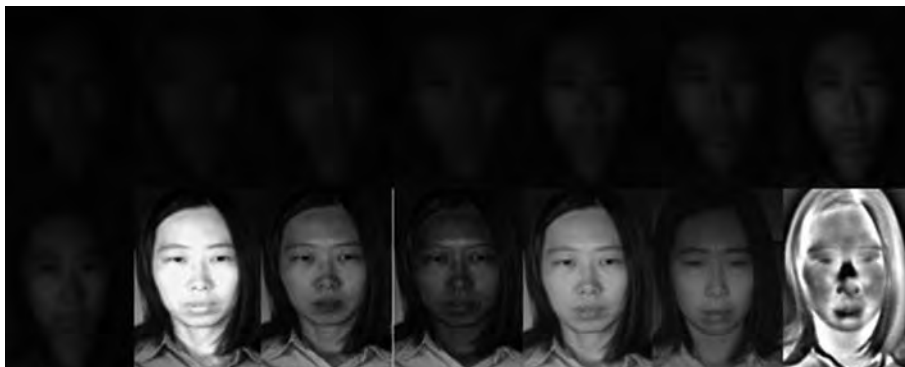
Multispectral and Hyperspectral Biometrics. Figure 3 A set of multispectral face images acquired in 8 single narrow bands of the visible spectrum, followed by the three R, G, B components from a conventional color camera, the composite color image, a NIR, and a thermal infrared image of the same subject- (Courtesy of Imaging, Robotics, and Intelligent Systems lab, University of Tennessee).
