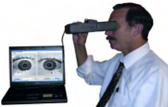
Iris Acquisition Device. Figure 8 An example of the ISCAN2 (from http://www.crossmatch.com/I_SCAN_2.html ).
