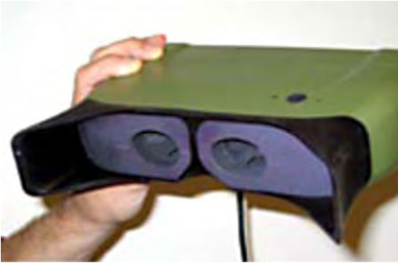
Iris Acquisition Device. Figure 11 An example of the MobileEyes (from www.retica.com ).
