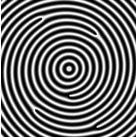
Fingerprint Sample Synthesis. Figure 3 A simple synthetic pattern generated by equations (1)–(3), with \varphi_0(x, y) = 20 \cdot 2\pi \cdot \sqrt{x^2 + y^2} and \{(x_i, y_i)\} = \{(0.2, -0.25), (-0.2, -0.37), (0.0, 0.2), (-0.25, 0.3), (0.2, 0.43)\} .
