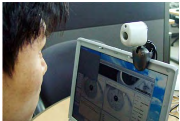
Iris Acquisition Device. Figure 10 An example of the JIRIS1000 (from http://www.engadget.com/2006/03/06/jiris-jpc1000-brings-iris-scanning-home/ ).
