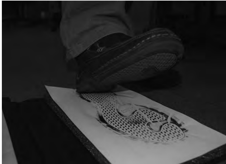
Footwear Recognition. Figure 2 Making an outsole pattern print on sensitized paper with the Printscan method.
