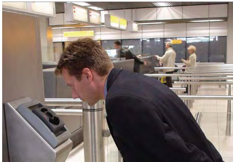
Iris Recognition at Airports and Border-Crossings. Figure 2 At Schiphol Airport (Amsterdam NL), the Privium Program has a membership of about 40,000 frequent travelers. They pay an annual fee to use the iris recognition system at automated gates, thereby avoiding the queues at Immigration for passport presentation.
