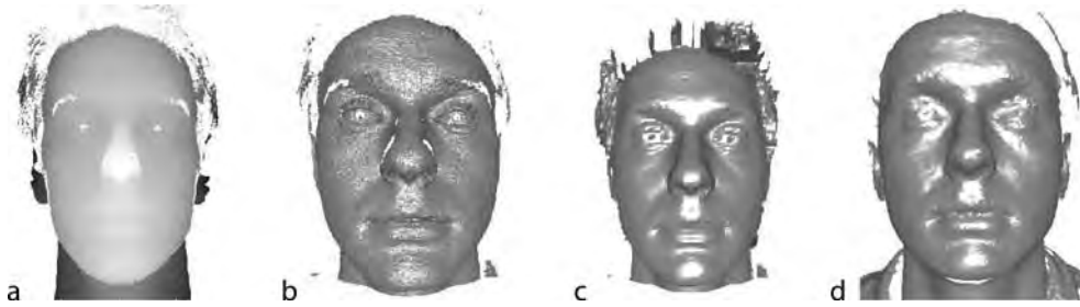
Face Recognition, 3D-Based. Figure 2 Sensor-dependent preprocessing. Laser range scanner: (a) input depth image, (b) raw polygonal data (200,000 triangles), and (c) processed data (16K). Stereo camera: (d) raw data (34,000 triangles).
