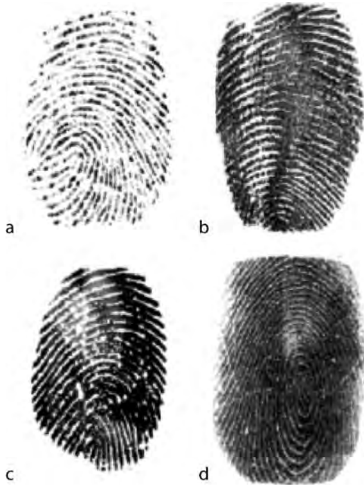
Liveness Detection: Fingerprint. Figure 1 Example of live and non-live fingerprints captured by Capacitive DC scanner: (a) live finger; (b) spoof finger made from Play-Doh; (c) spoof finger made from gelatin; (d) cadaver finger.
