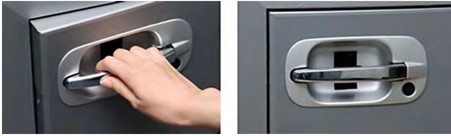
Finger Vein Reader. Figure 2 Finger vein reader embedded on a door handle.
