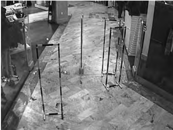
Gait, Forensic Evidence of. Figure 1 Measuring screens put up in a department store, in order to calibrate the CCTVs [10].
