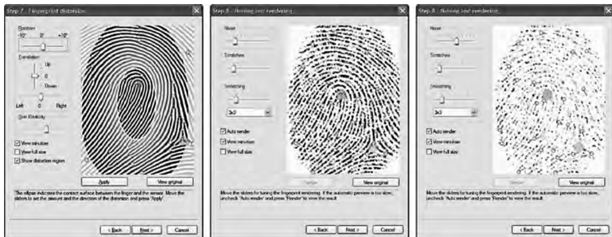
SFinGe. Figure 6 Graphical user interface for fingerprint distortion (left) and noising (middle and right).
