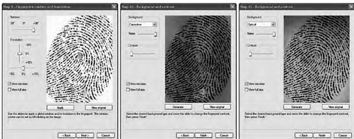
SFinGe. Figure 7 Graphical user interface for global rotation/translation (left) and background generation (middle and right).
