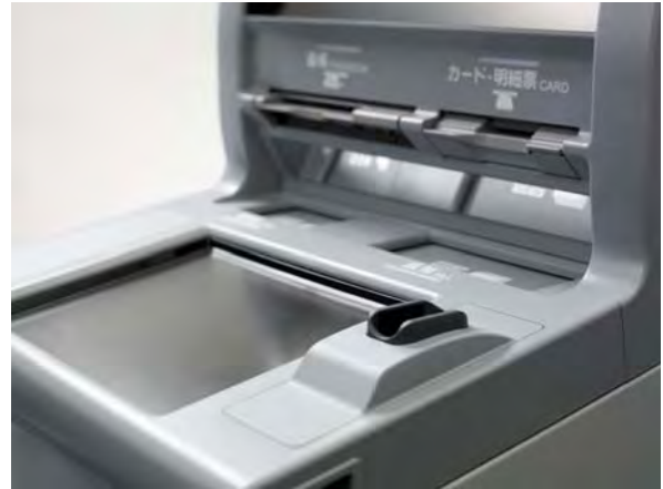
Finger Vein Reader. Figure 1 Finger vein reader implemented on an ATM.
