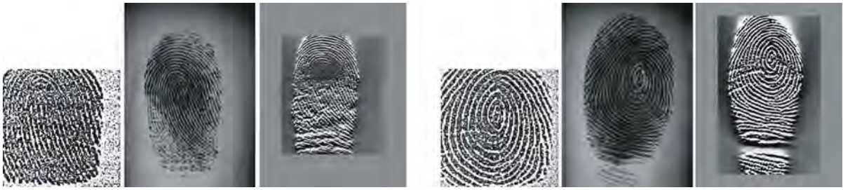
Fingerprint Databases and Evaluation. Figure 2 Example fingerprint images of two fingers acquired with three different sensors (from the BioSec baseline corpus). Fingerprint images of the same finger are shown for a capacitive sensor ( left of each subplot ), an optical sensor ( center ) and a thermal sensor ( right ).
