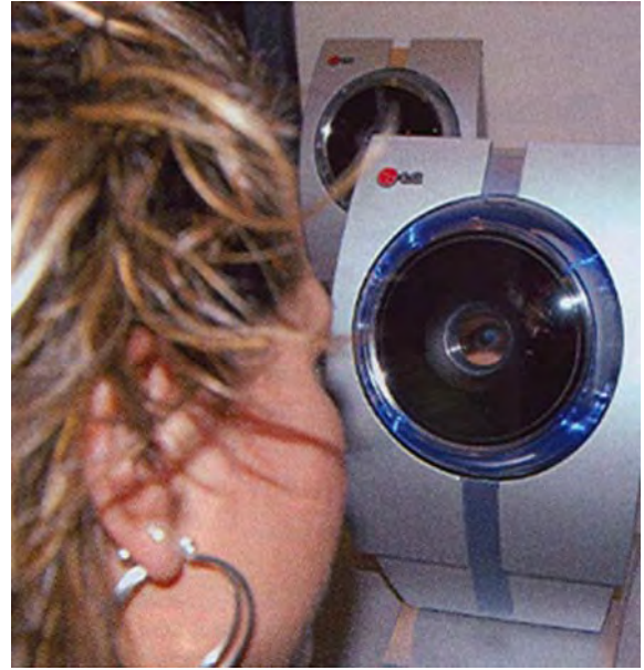
Iris on the Move™. Figure 1 An enrollment quality iris image capture device, the LG IrisAccess 3000. (Photo provided courtesy of Mohammed Murad of LG Electronics USA Inc., Iris Technology Division.)
