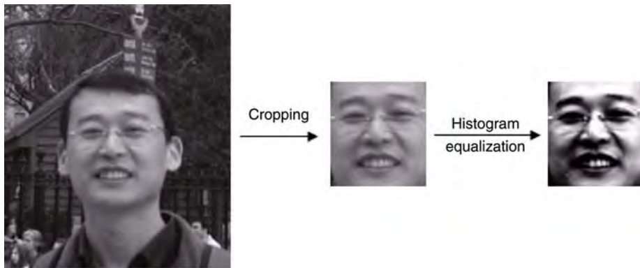
Image Pattern Recognition. Figure 2 Image cropping and histogram equalization.
