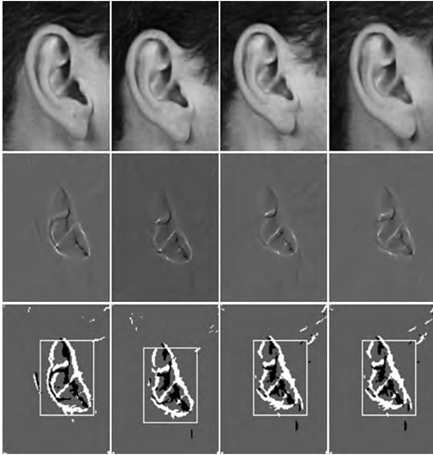
Physical Analogies for Ear Recognition. Figure 3 Feature extraction for subject 000, row: (a): 141 \times 101 ear images, row (b): Convergence fields, row (c): Thresholded convergence maps.
