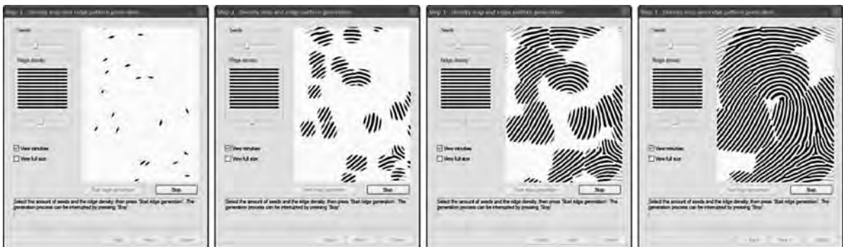
SFinGe. Figure 4 Graphical user interface for the ridge-line pattern generation.
