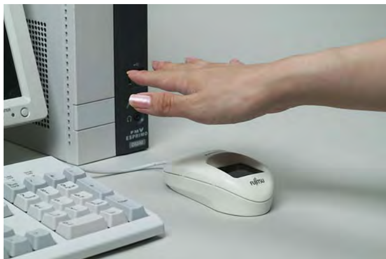
Palm Vein Image Sensor. Figure 2 PC mouse equipped with palm vein authentication sensor.
