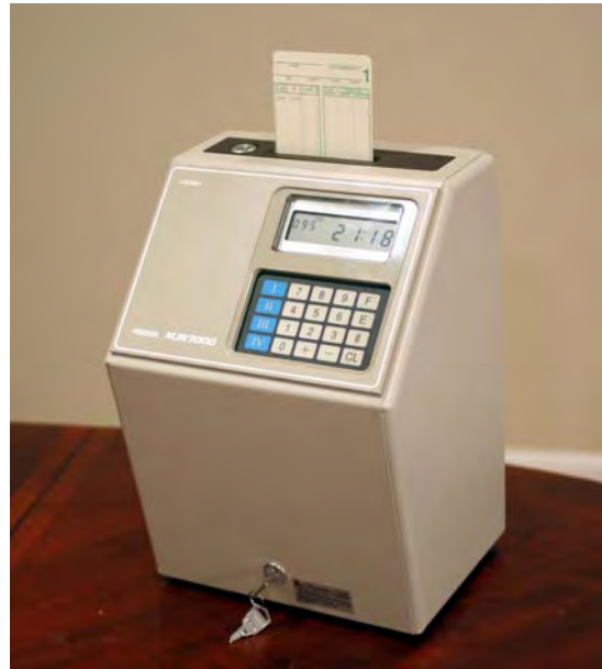
Time and Attendance. Figure 1 Typical punchcard based time clock.
