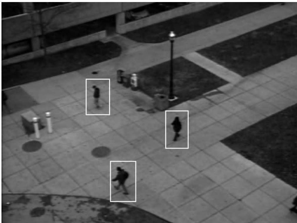
Human Detection and Tracking. Figure 1 Typical human detection output showing the location and scale of people.
