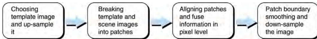
Iris Super-Resolution. Figure 2 The flow chart of the iris Super-Resolution algorithm.
