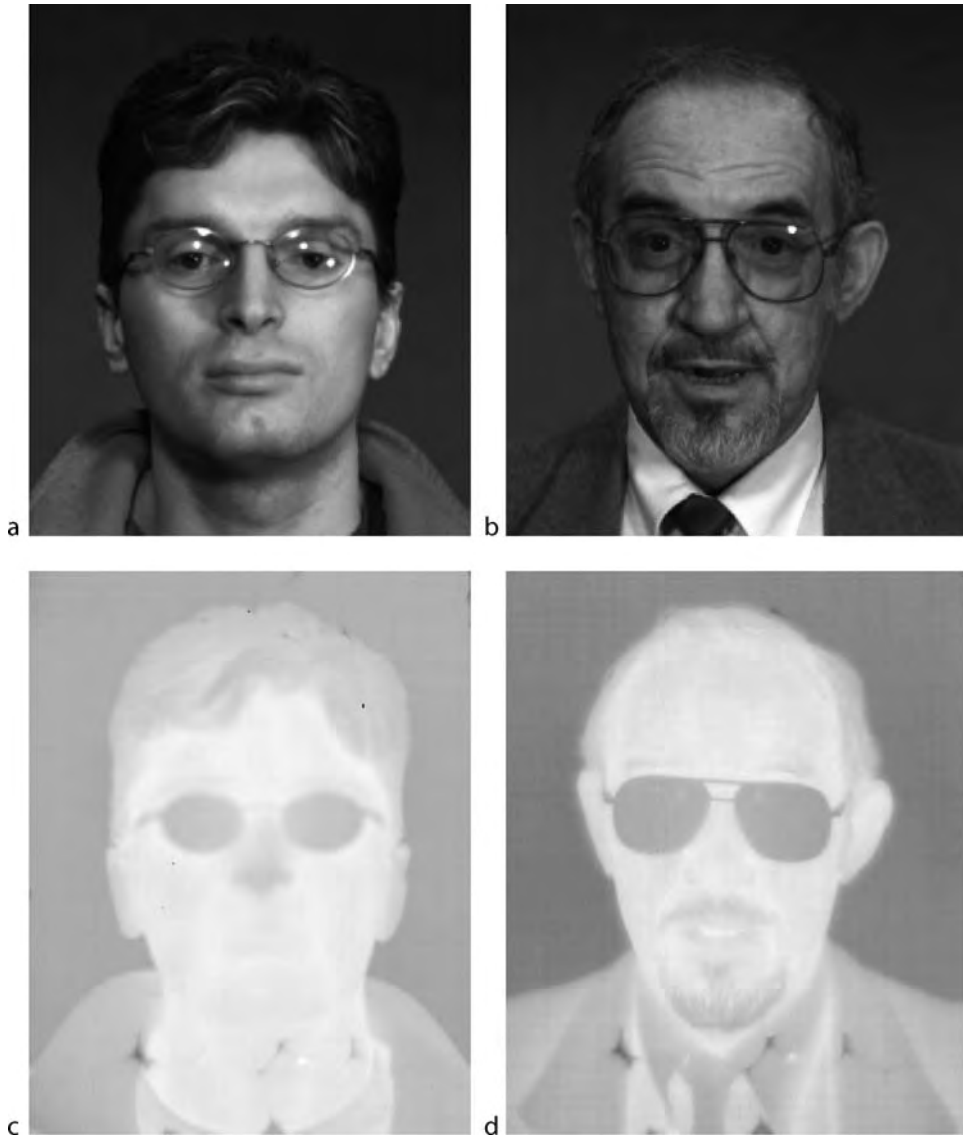
Face Recognition, Thermal. Figure 2 (a, b) Visible images; (c, d) thermal IR images. It should be observed that since thermal IR is opaque to glass, the presence of eyeglasses blocks the eyes completely.
