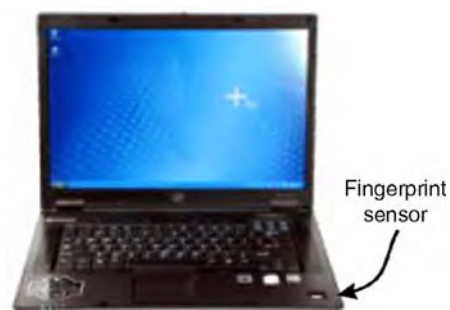
Biometric Sample Acquisition. Figure 3 Fingerprint Sensor in Laptop computer
