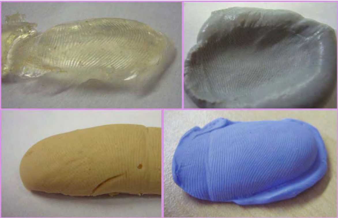
Fingerprint Fake Detection. Figure 5 Some moulded fakes: gelatine, plastic (negative), alginate, silicon.
