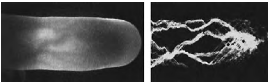
Finger Vein Biometric Algorithm. Figure 1 Visualised finger vein network (left) and its segmented pattern (right).
