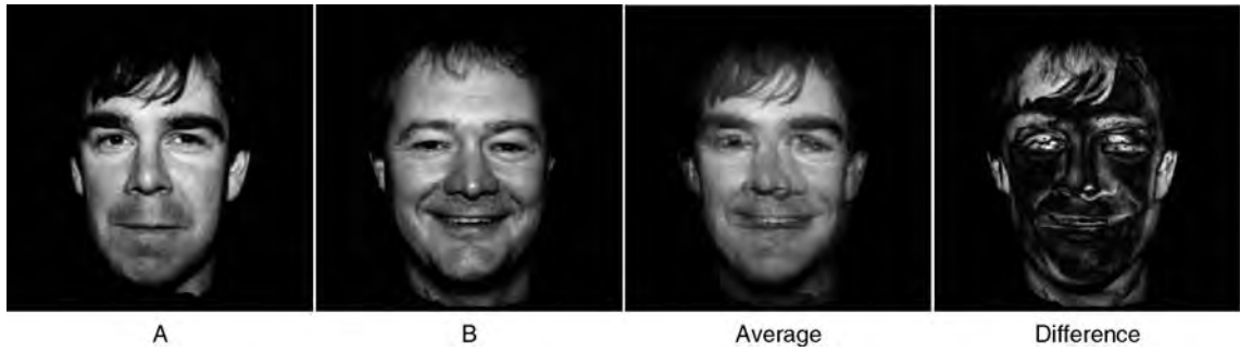
Face Alignment. Figure 1 To compare two face images, by directly adding them or subtracting one from another does not produce the desired result. Face alignment enables to establish correspondences between different images, so that the subsequent tasks can be performed on a common basis.
