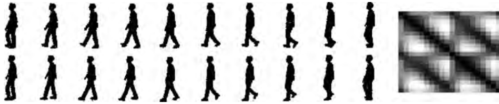
Gait Recognition, Motion Analysis for. Figure 1 Twenty sample frames from a walking cycle from a side view. Each row represents half a cycle. Notice the similarity between the two half cycles. The right part shows the similarity plot: each row and column of the plot corresponds to one sample. Darker means closer distance and brighter means larger distances. The two dark lines parallel to the diagonal show the similarity between the two half cycles.
