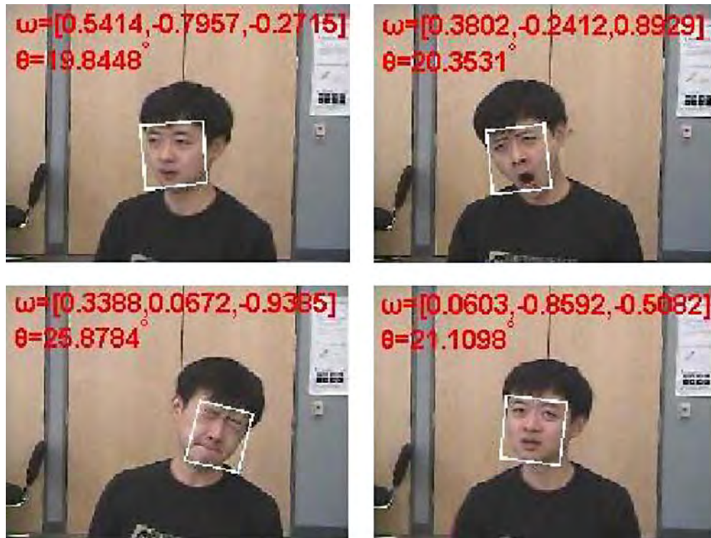
Face Tracking. Figure 2 An example of face tracking under changes of pose and expressions. The estimated pose is shown on the top of the frames. The pose is represented as an unit vector for the rotation axis, and the rotation angle in degrees, where the reference is taken to be the frontal face.
