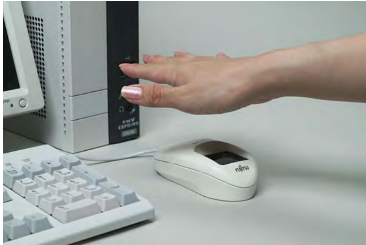
Palm Vein. Figure 4 PC mouse containing palm vein authentication sensor.
