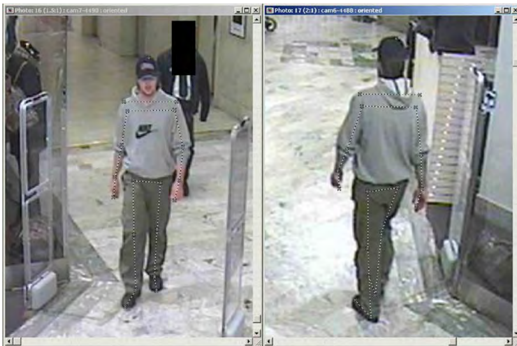
Gait, Forensic Evidence of. Figure 2 Screen shots of PhotoModeler Pro ® interface, showing selection of points. Simultaneous images from different CCTV cameras are used to pinpoint concurrent anatomical points (and markers) seen from different POV. The lines between the points are to scale and thus hold accurate measures of distance [10].
