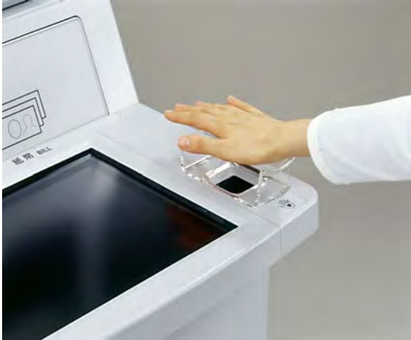
Palm Vein Scanner. Figure 3 ATM with palm vein authentication sensor.
