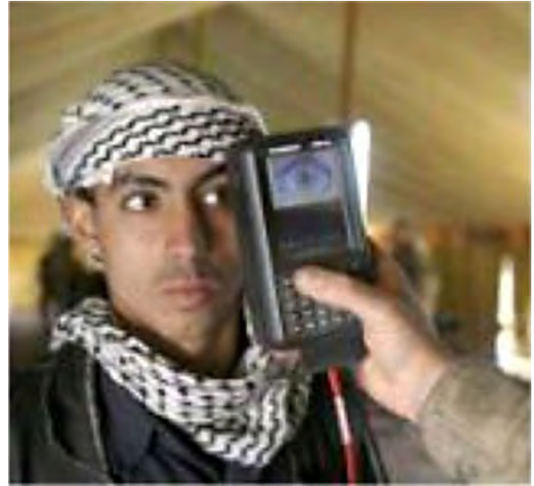
Iris Acquisition Device. Figure 12 An example of the PIER 2.3 (from http://www.securimetrics.com/solutions/pier.html ).
