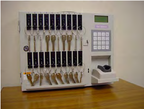
Finger Vein Pattern Imaging. Figure 9 Key management system with a finger vein reader (Courtesy of Hitachi-Omron Terminal Solutions, Corp.) Metal enclosure is removed for demonstration purpose.
