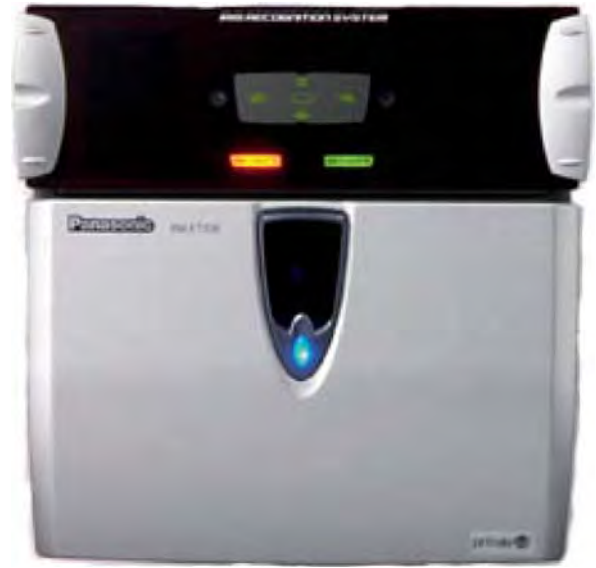
Iris Acquisition Device. Figure 2 An example of the Panasonic BM-ET 330 (from http://panasonic.co.jp/pss/bmet330/en/ ).
