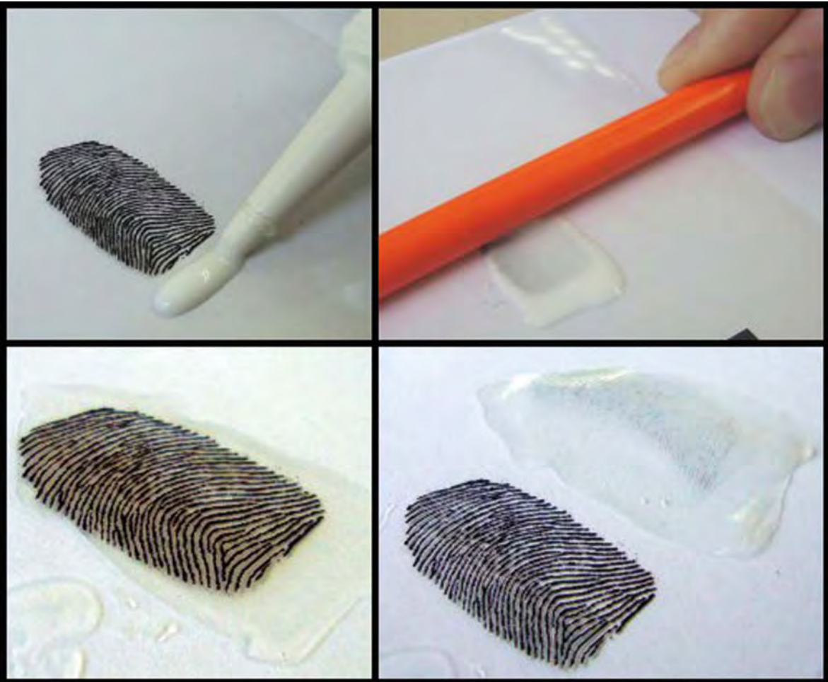
Fingerprint Fake Detection. Figure 3 Wood glue using a printed fingerprint as negative.
