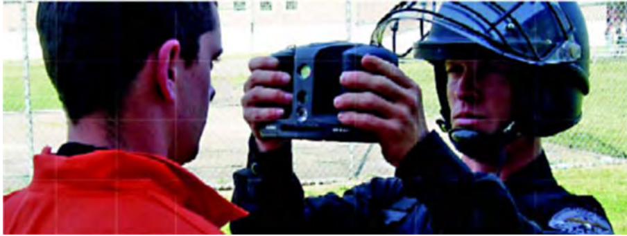
Iris Acquisition Device. Figure 3 An example of the L-1 HIDE Series 4 (from http://www.llid.com/images/stories/solutions/hiide_product_sheet.pdf ).
