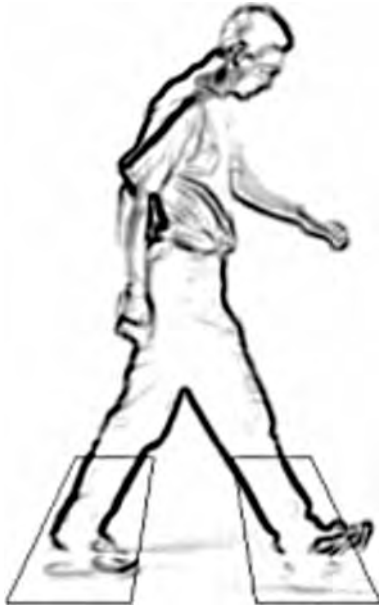
Gait Recognition, Model-Based. Figure 5 Binary mask to detect gait cycle. The sum edge strength within the mask varies periodically during the subject's gait and the heel strike being the greatest.
