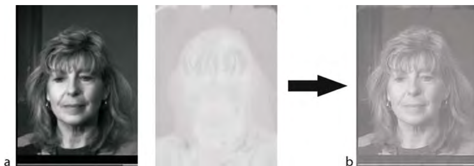
Fusion, Sensor-Level. Figure 3 Multi-spectral face image fusion. (a) Visible and infrared spectrum images and (b) Fused image.
