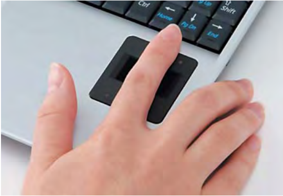
Finger Vein Pattern Imaging. Figure 11 Bottom-lighting system (Hitachi Laptop PC Se210) (Courtesy of Hitachi, Ltd.).
