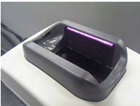
Finger Vein Pattern Imaging. Figure 6 Infrared LED array (Courtesy of Hitachi-Omron Terminal Solutions, Corp.) Infrared LEDs are colored in this picture for visualization.
