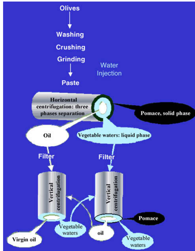
Figure 9.2: Flow diagram of the olive oil extraction process. Source: Unctad ( www.unctad.org (2004)).
