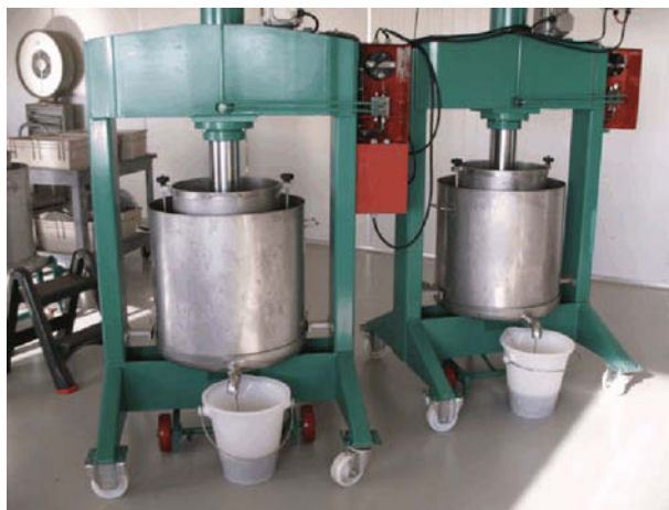
Figure 8.6: Olive oil content determination by mechanical method.
