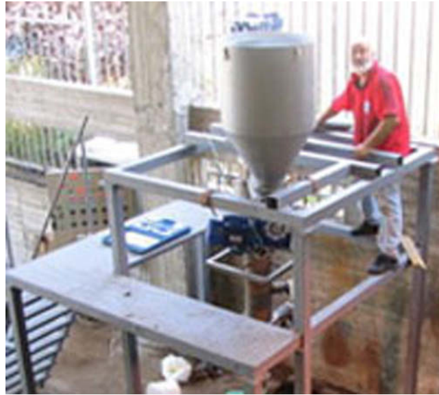
Figure 12.6: A bioreactor for producing methane from olive-mill waste, developed by Dr Yuri Wladislavsky.
