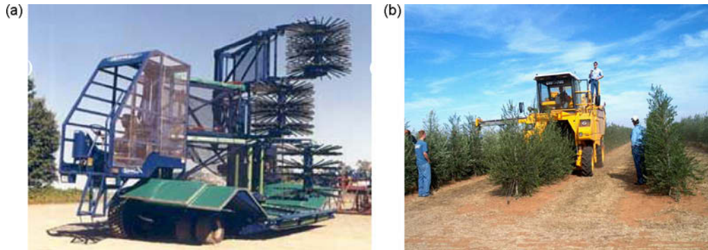
Figure 8.18: (a) Side-pass comb harvester; (b) straddle harvester.
