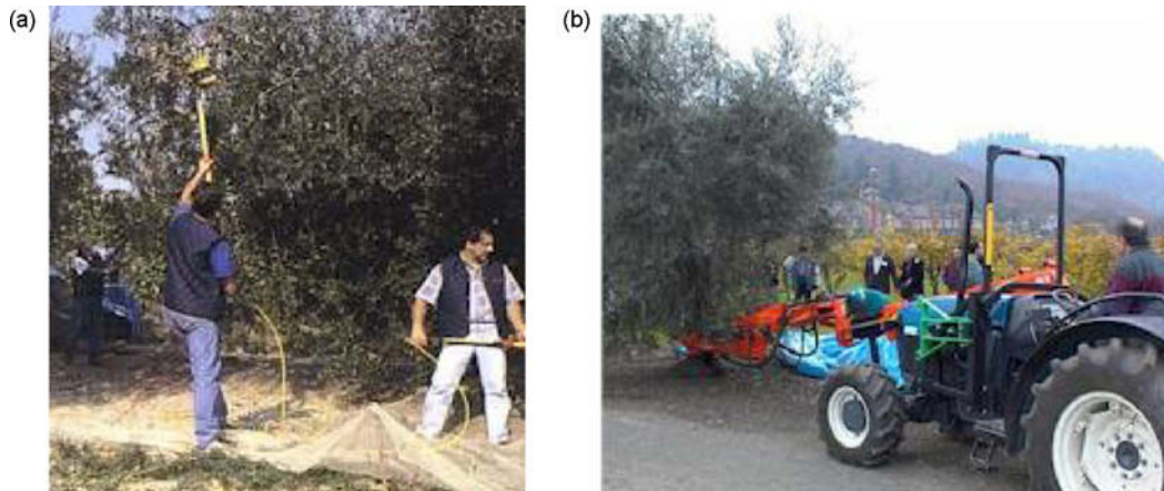
Figure 8.17: (a) Hand-held pneumatic comb; (b) tractor-mounted shaker. Source: TDC-Olive (2004).
