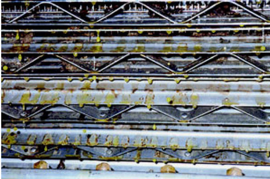
Figure 9.4: Percolation of the olive oil from the olive paste in a Sinolea unit.
