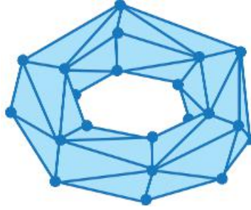
Figure 1.45 Up to homeomorphism, a torus can be triangulated as a simplicial complex.
