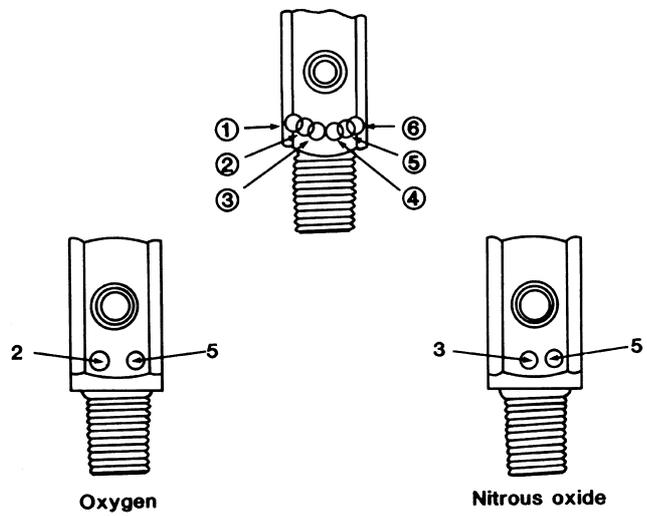
**Figure 5-1** Diagram of the pin index safety system, illustrating the spacing between the valve outlet and pin holes in the valve bodies for oxygen and N<sub>2</sub>O cylinders. The numbering system identifies each pin hole site. (Reprinted with permission from CE Short, *Principles and Practice of Veterinary Anesthesia*, Baltimore: Williams & Wilkins, 1987, page 397.)
