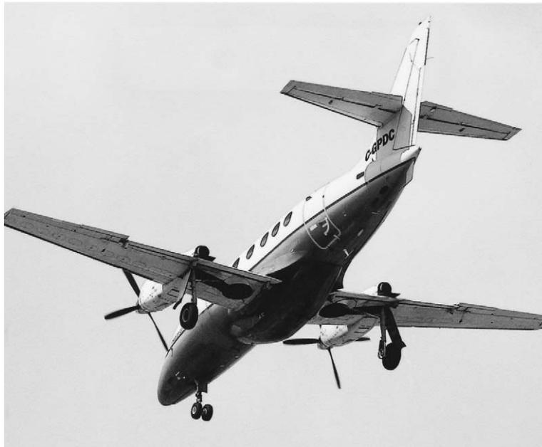
**Figure 4-1** • A small, twin-engine commuter on final approach, with flaps and landing gear down, exemplifies the modified elliptical wing shape typical of many such aircraft.
