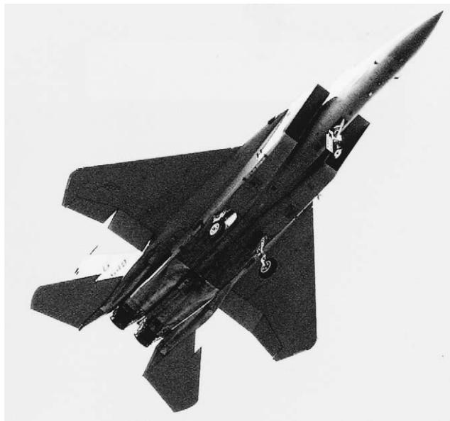
**Figure 4-2** • The short triangular wings of an F-15 Eagle, as seen from below, are characteristic of a Mach 2.5 air-superiority fighter.
