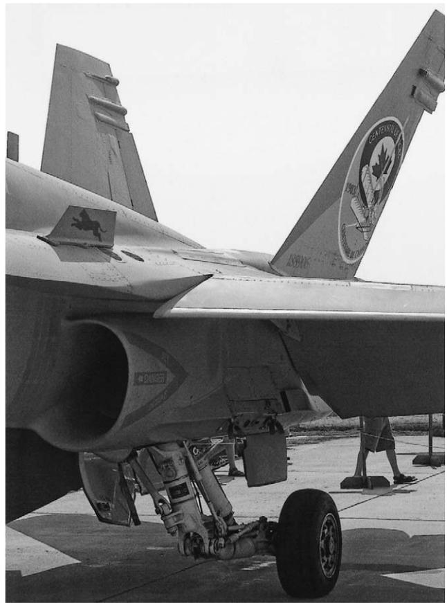
**Figure 4-11** • Dual tail fins characterize the tail of most modern-day supersonic fighters, in this instance an F-18 "Hornet."
