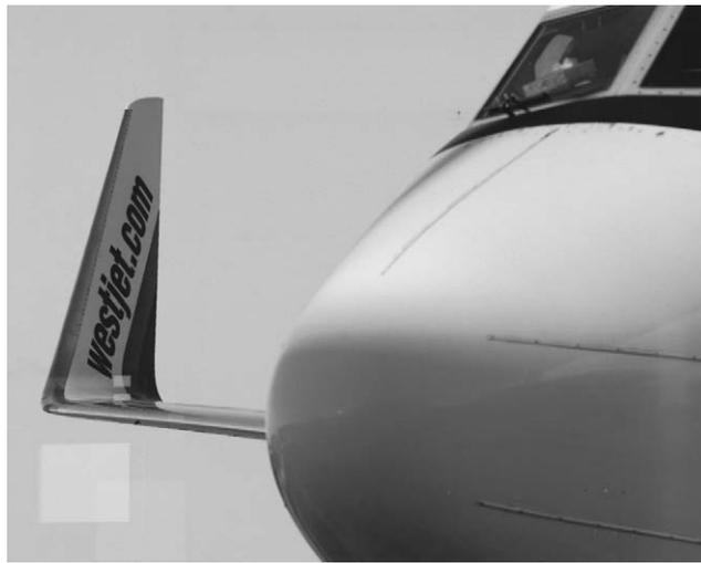
**Figure 4-7** • Most modern jetliners now come equipped with winglets, which are small fins situated at the end of each wing that help the aircraft resist stalling.
