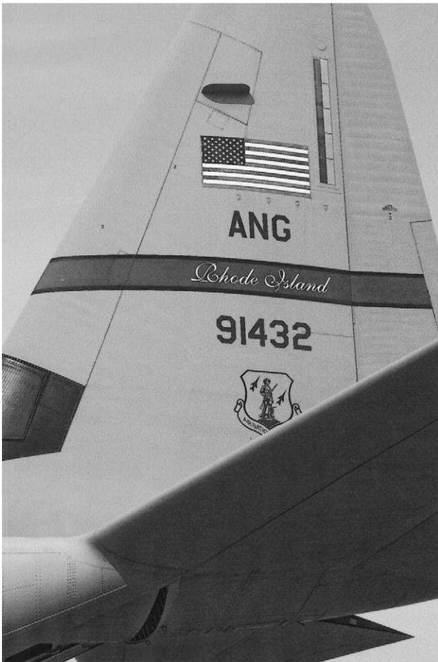
**Figure 4-10** • Single vertical stabilizer and rudder of a C-135 refueling aircraft.
