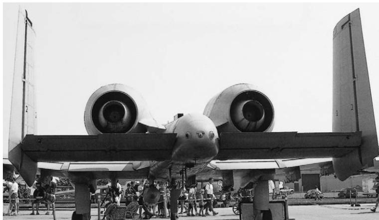
**Figure 4-12** • An A-10 "Warthog" viewed from behind shows its striking engine nacelles flanked by a pair of large tail fins.
