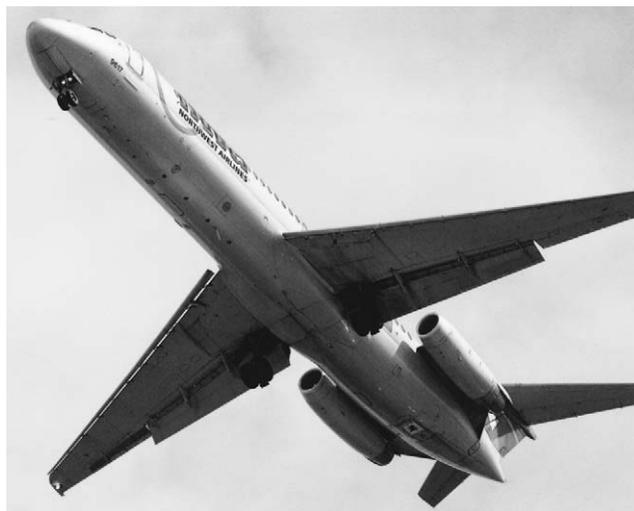
**Figure 4-6** • A jet airliner on its final approach has deployed both its leading edge slats and trailing edge flaps to increase its lift so that it may reduce its thrust and thus decrease its landing speed.
