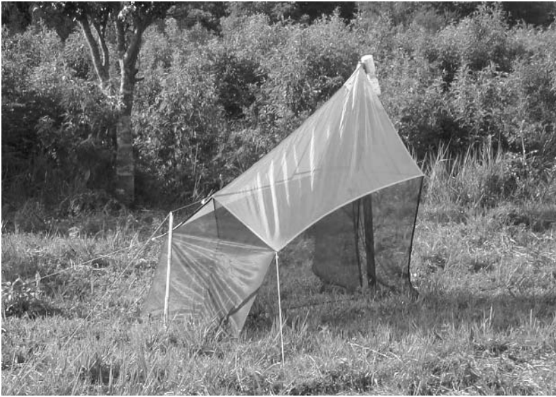
Fig. 33.4. Version of the Malaise trap (Malaise, 1937) with white roof and black walls, deployed at pasture edge. (Martin Hall.)
