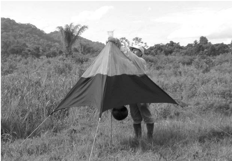
Fig. 33.3. Version of the canopy trap (Catts, 1970), with spherical black 'target' suspended under the canopy, being deployed in Bolivia. (Martin Hall.)
