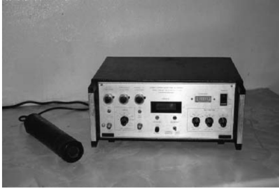
Fig. 17.30 Point probe gamma scintigraphy scanner, with lead-collimated hand-held point probe and counter.
