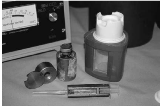
Fig. 17.32 Equipment used for delivery of gamma-emitting radioisotope. The syringe is encased in a tungsten alloy shield. The vial of radioactive solution is shielded in a lead container (left) or purpose-designed eluting jar (right). Note the appropriately calibrated Geiger-Müller counter in the background.
