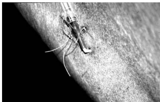
Fig. 13.7 A kinked polyurethane catheter.
