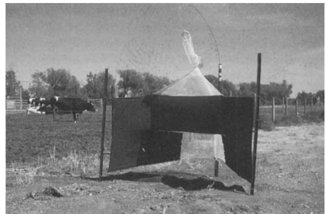
Figure 6-9. A tsetse fly trap designed by scientists at ICIPE in Nairobi, Kenya. Traps such as these can be built and maintained by villagers who have a stake in tsetse fly control to reduce the occurrence of trypanosomiasis in humans and livestock. (Photo courtesy of Dr. Steve Mihok)
