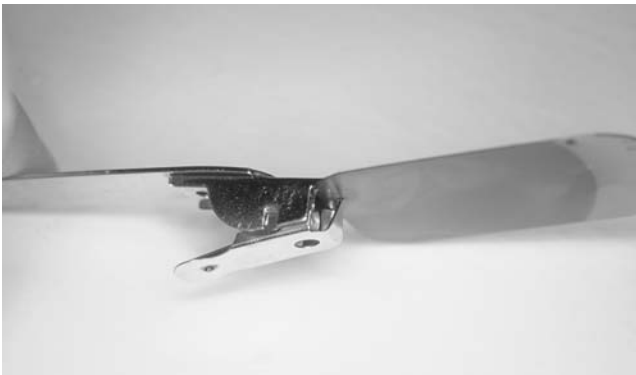
FIGURE 4.55. Film hanger attached to film.
