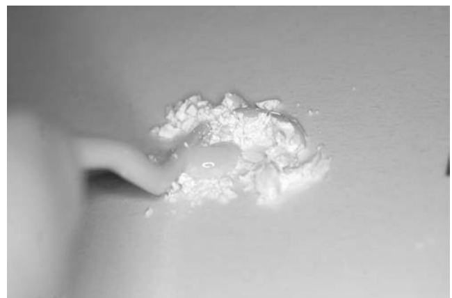
FIGURE 8.29. Using a spatula to mix the liquid and powder.
