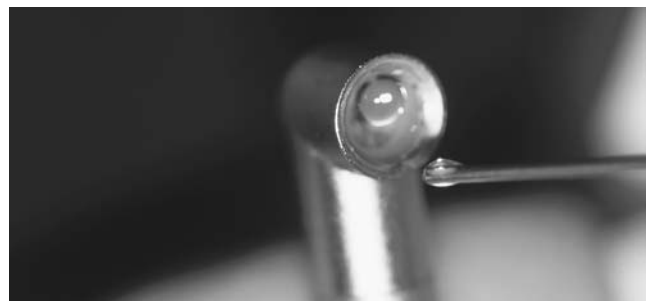
FIGURE 2.157. Application of oil to head of polishing angle.
