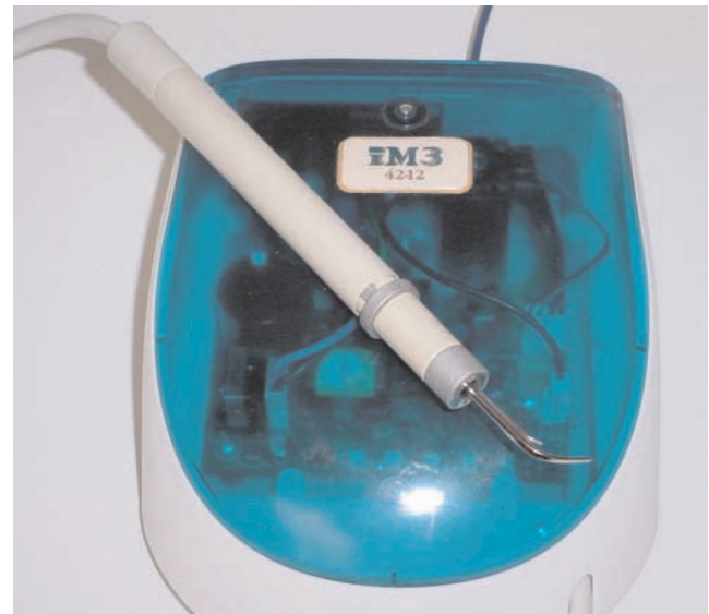
FIGURE 2.97. Ferrite rod ultrasonic scaler—iM3 Model 42-12.
