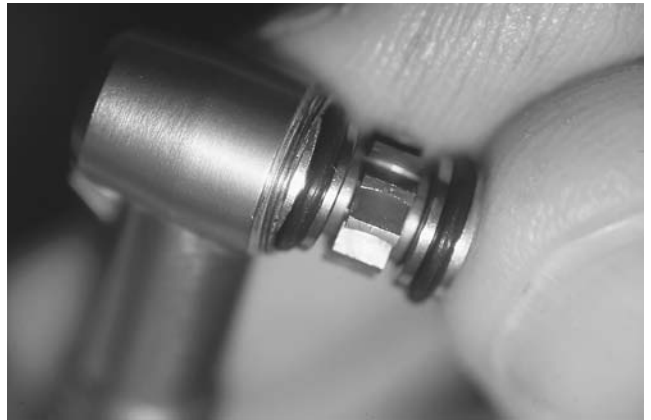
FIGURE 2.152. Snapping turbine into handpiece head.
