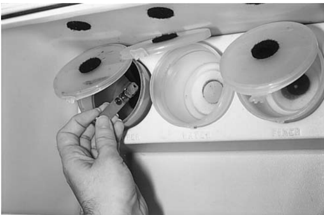
FIGURE 4.56. Looking down into the chairside darkroom, exposed film is manually inserted in developer container.
