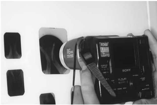
FIGURE 11.9. Camera position for digitized radiographic survey.
