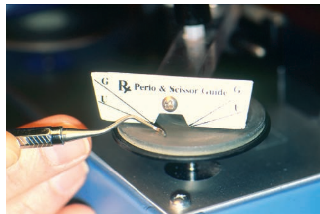
FIGURE 2.85. Mechanical instrument sharpener. (Rx Honing Machine Corporation, Mishawaka, IN)
