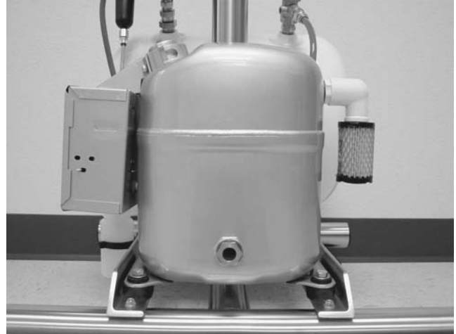
FIGURE 1.22. Silent compressor connected to the delivery system cart (iM3).
