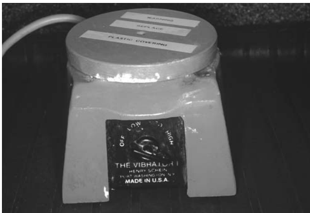
FIGURE 9.19. Vibrator to mix dental stone.
