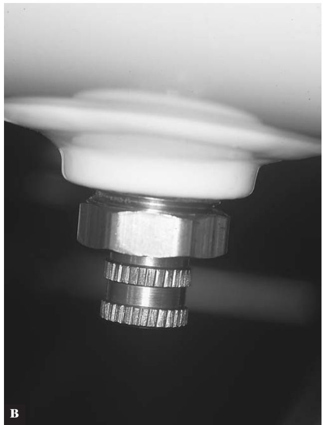
FIGURE 2.159. Screw device used to empty condensation from air tank (im3).
