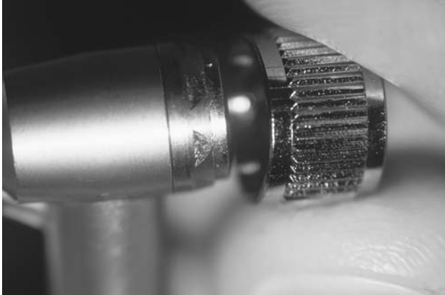
FIGURE 2.148. Turbine removal tool used to unscrew the turbine cover.
