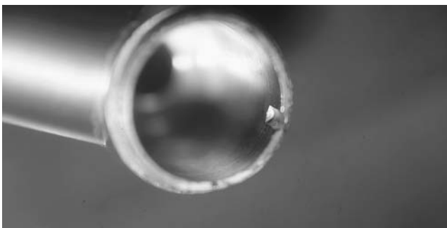
FIGURE 2.150. Handpiece head without turbine (note indented space for turbine).
