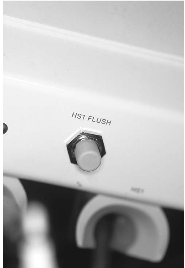
FIGURE 2.164. Chlorhexidine flush for iM3 lines and handpieces.
