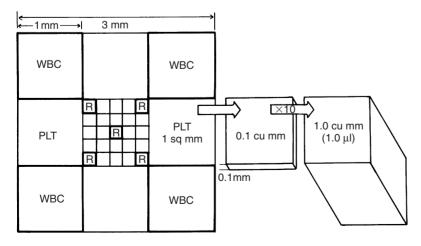
FIGURE 2-2. Dimensions of a hemocytometer. The hemocytometer grid consists of 9 mm². The central 1 mm² is additionally divided into 25 squares. The areas usually used for erythrocyte, leukocyte, and platelet counts are indicated by R, WBC, and PLT, respectively. Because the hemocytometer is 0.1 mm deep, the cells counted over 1 mm² are in the volume of 0.1 mm³. To determine the cells in 1 mm³ (which is 1  $\mu$ l), one should multiply by 10.
