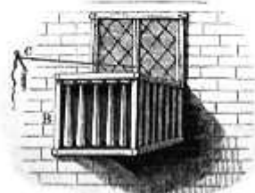
Trap of Pigeon-loft. Interior showing the loose bars called "the bolt." B, the little swinging doors on the inner end, C, the string which pulls up the outer door.
