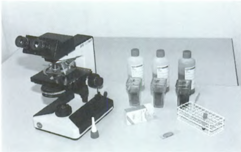
Fig. 5 A good quality high power microscope is an important tool in every diagnostic laboratory. A standard equipment should contain the following magnifications: 32 × 100 ×, 400 × and for the investigation of blood smears 1000 × with oil immersion. Rapid staining methods for blood smears are of great practical use in the routine diagnostic laboratory. The previously air-dried smears are fixed and stained in only 15 s by three consecutive brief immersions in the pre-prepared staining solutions.
