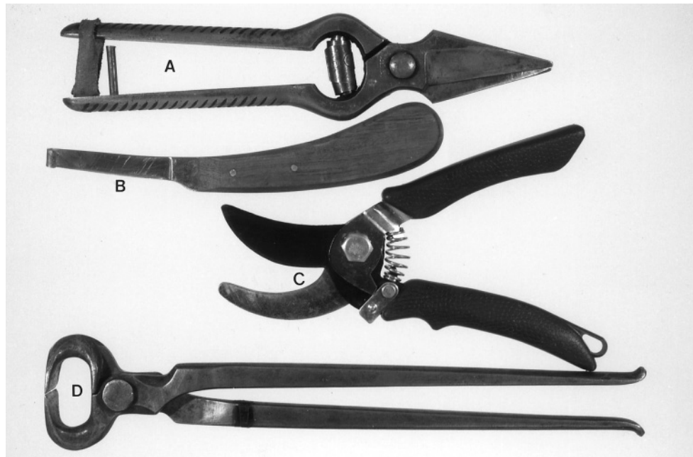
Figure 10.30. Hoof-trimming tools. (A) Burdizzo sheep nail trimmer, (B) hoof knife, (C) pruning shears, (D) equine hoof nipper.
