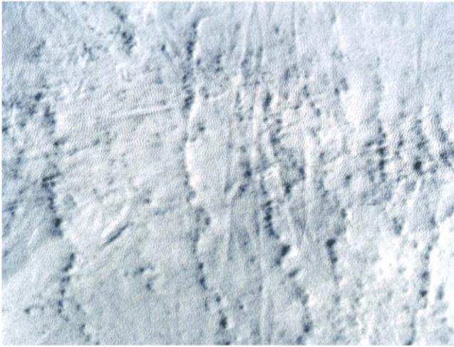
FIGURE 17.10 Feeding damage caused by the sheep ked, Melophagus ovinus (Hippoboscidae). Grain side of pickled sheepskin showing pitted surface, or cockle. (Courtesy of USDA.)
