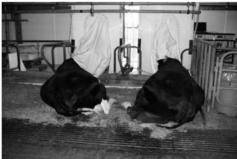
Fig. 10.2. Cows in the ventilated head-hoods during measurement of gaseous exchange (lying down).
