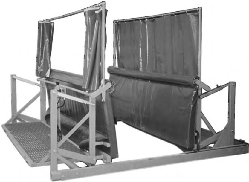
Fig. 17.5. (a) A hydraulically operated deer handler shown in its open position; this creates a small padded room about 1.4 \times 2.6 m long which is suitable for holding one or two deer. The curtains are closed during loading but can be opened after the animal(s) has (have) been restrained. The operator works from the small platform and restrains an animal by operating the moving wall, and applying steady pressure to the animal aligned between the two walls. ( Continued overleaf. )
