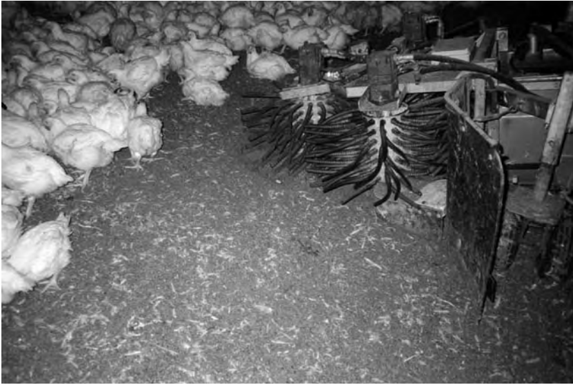
Fig. 18.3. Poultry-catching machine. The rotating heads with soft rubber fingers are mounted on the end of a long, pivoting boom. This provides the operator with more precise control because he/she can control both sideways and forward movement of the machine. To enable the operator to observe chickens more closely during pick-up, he/she stands next to the pick-up head and operates the machine with a controller that he/she carries.
