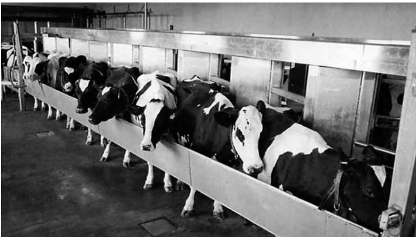
Fig. 8.4. Herringbone rapid-exit brisket bar. The straight, rapid-exit brisket bar in a herringbone allows cows and heifers of various sizes to be milked together with ease and maximum comfort. Longer cows slide along the bar. Heifers may adapt more easily to being milked in a herringbone. Cows of varying age, size and infirmity may have difficulty making the sharp turn into a parallel milking centre (photograph courtesy of DeLaval, Inc.).
