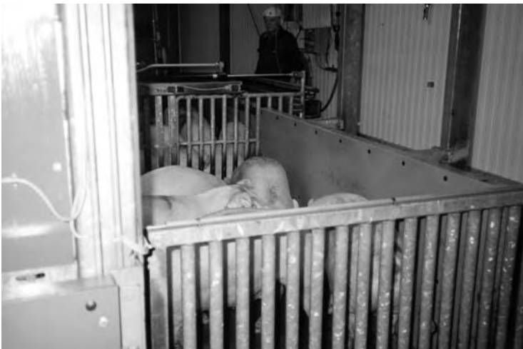
Fig. 20.6. Danish group handling system for moving groups of five pigs into a CO 2 chamber.
