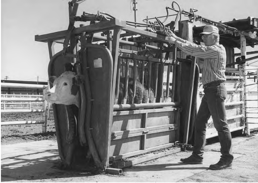
Fig. 7.6. Hydraulically operated squeeze chute (crush). When the pressure is properly set, a hydraulic squeeze is safer because protruding lever arms are eliminated. The pressure should be set so that squeezing will automatically stop before cattle bellow or strain.
