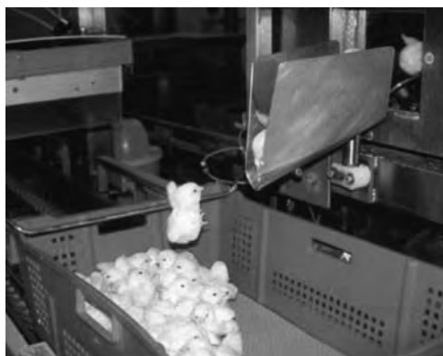
Fig. 18.2. Automated chick-counting into transport crate. Photograph courtesy of Dr Andrew Butterworth.
