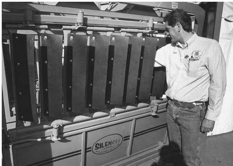
Fig. 7.7. Rubber louvres installed on the squeeze chute to prevent incoming cattle from seeing people. This will facilitate cattle entry into the chute.
