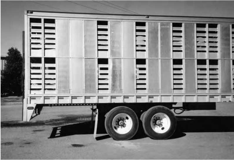
Fig. 15.7. Truck trailer for transporting pigs, with removable panels for adjustment of ventilation. More panels are added during cold weather but removed in summer. The panels are constructed from thin plastic and they slide into slots on the trailer.
