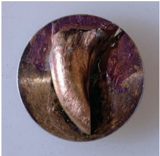
Figure 8.9 Gold spattering, a technique used in scanning electron microscopy work, in this case on the beak of a cockerel that was found following an alleged cock-fighting competition. (Courtesy of Richard Spence.)
