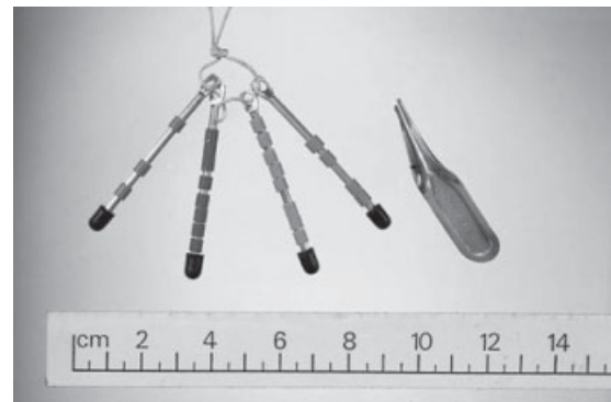
Figure 6.1 Coloured plastic rings, with metal applicator. Such rings are ideal for temporarily marking confiscated birds. This figure also appears in colour in the colour plate section.
