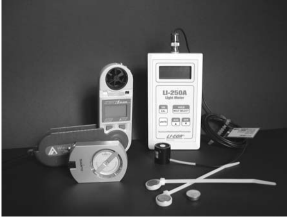
Fig. 5.5 A selection of instruments used by ecologists to record abiotic environmental conditions. From front in a clockwise direction: temperature loggers (plastic cable ties aid their location in the soil (Thermochron iButtons, manufactured by Dallas Semiconductors); clinometer (Suunto); hand-held wind meter, with built-in temperature and humidity sensors (AZ Instruments); light meter with sensor for measuring photosynthetically active radiation or light intensity (Li-Cor) (Courtesy Peter le Roux).
