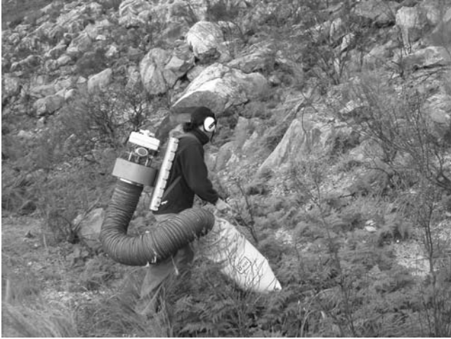
Fig. 4.11 Suction sampler in action, being used to sample insects from low-growing vegetation (Courtesy James Pryke).
