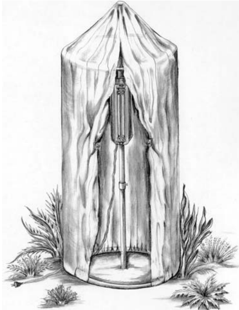
Fig. 4.17 Light tower. This is a tent made of a thin white sheet over a frame, with a light inside. The tent is closed during operation. Insects attracted to the tower rest on the outside and are collected by hand.
