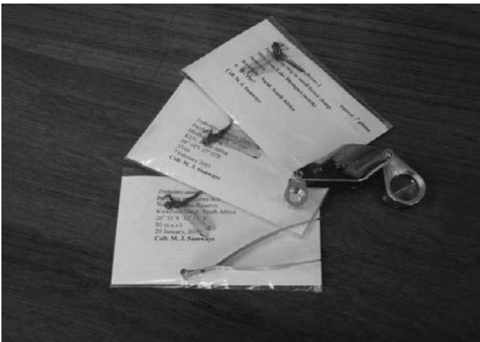
Fig. 2.10 Very sensitive forceps, home-made out of packing case steel, for handling delicate insects, e.g. putting in and taking out of dragonflies from transparent envelopes. Also shown is a simple but very versatile and useful piece of field equipment—a good-quality 10× and 20× hand lens.
