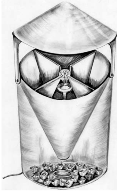
Fig. 4.16 Light trap with a roof to keep off rain and a mesh-covered plug hole to drain out any water that may enter the trap. Insects enter the funnel and are 'knocked down' by the vertical veins. Pieces of egg box at the bottom of the trap give the insects something on which to sit. Although shown here as transparent, the trap is normally made of a material such as aluminium.
