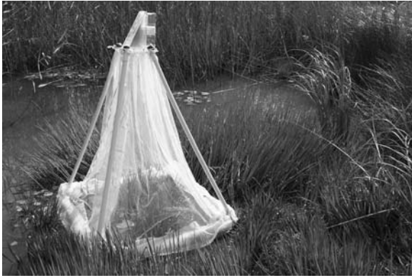
Fig. 4.31 Aquatic emergence trap, being used here to sample emerging adult insects. As the insects leave the water to become adults, they fly up to the top of the tent where they are directed by a Perspex funnel into a chamber made out of two plastic jars facing each other, with a hole cut into the side of the top one. If the insects need to be kept alive, no preservative is placed in the chamber. Otherwise, a preservative such as 70% ethanol is introduced. (Courtesy John Simaika).
