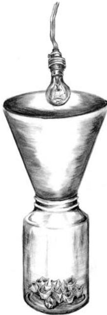
Fig. 4.15 Simple, portable light trap, made of a card cylinder inserted into a jar with pieces of an egg box in the bottom on which the captured insects can sit.
