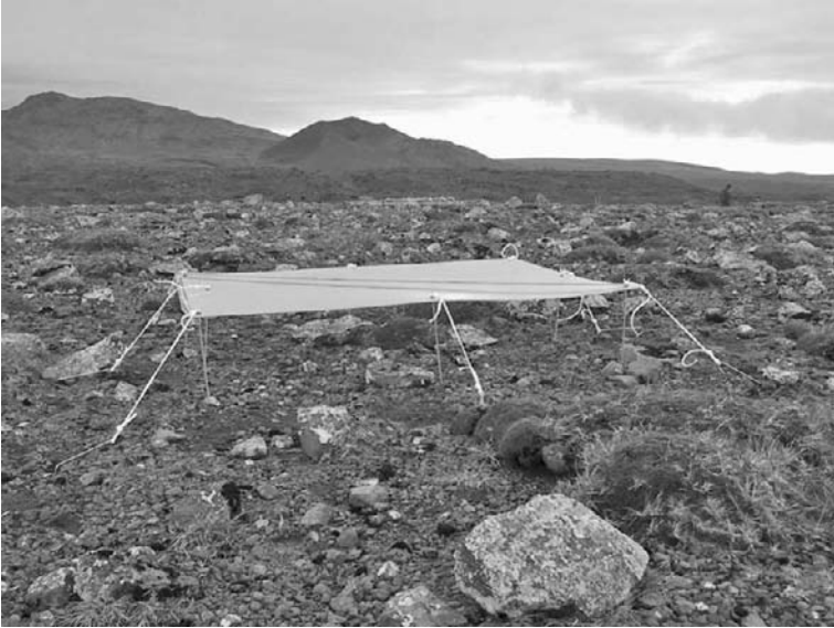
Fig. 11.1 A rain-out shelter (or cloche) made from transparent polycarbonate and used to dry and warm the local environment over cushion plants on sub-Antarctic Marion Island, and to quantify the response of the mite and springtail species inside the plant clump to climate change-related drying and warming (Le Roux et al. 2005; McGeoch et al. 2006).
