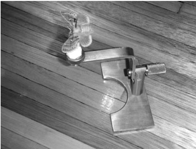
Fig. 2.15 An examination stage can be made by a local metal worker. The aim is to provide a stage on to which the insect is pinned for close examination, particularly under a binocular microscope, by turning through the vertical axis (with the lower knurled knob) and through the horizontal axis (with the upper knob).
