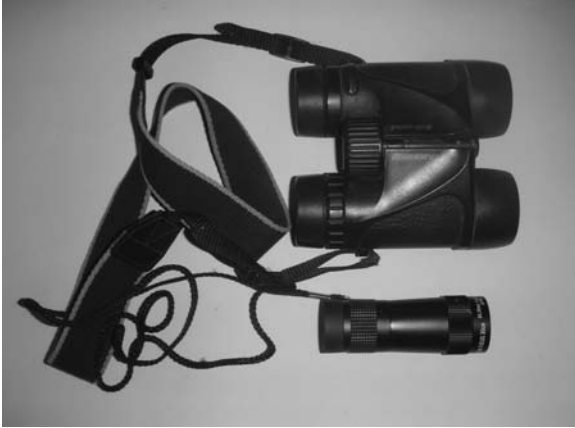
Fig. 4.24 The insect conservationists' two best friends: close-focus binoculars and a monocular. When in the shop choosing one of these, do make sure that you can focus on your toes while standing. Very few binoculars can focus this closely, so you will probably need to test several pairs. The ones shown here are lightweight 8×32 Kamakura, and have given years of service often under gruelling conditions. The monocular is an Opticron 8×20 Very Near Focus, and handy to have in your pocket for emergency use when you spot an interesting-looking insect while out on a family picnic.
