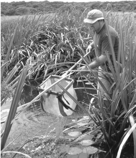
Fig. 4.30 Dip net used for catching aquatic arthropods: it must have a sturdy frame and tough gauze (Courtesy Ricky Taylor).
