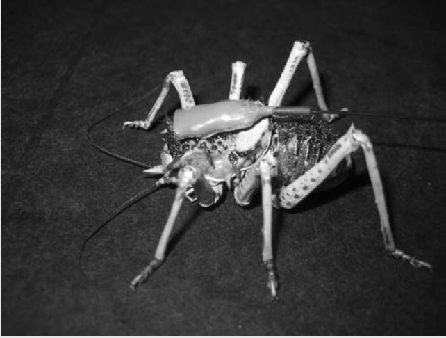
Insect with RT device for recording body temperature (Holohil Systems, Canada) attached to a king cricket (Orthoptera: Stenopelmatidae) (photo J.S. Terblanche).
