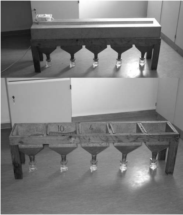
Fig. 4.29 (Upper panel) Bank of Berlese–Tullgren funnels with a series of six 60 W light bulbs above each funnel. (Lower panel) Bank of funnels with the canopy holding the light bulbs removed to show the funnels and the collecting bottles at the base containing 70% ethanol underneath (Courtesy James Pryke).
