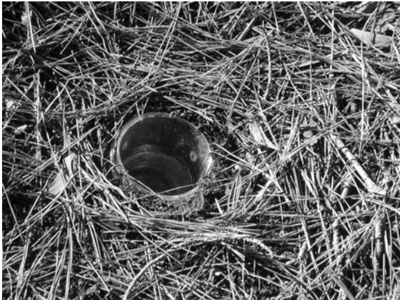
Fig. 4.27 Large-diameter pitfall trap that catches a wide variety of insects and other surface-foraging arthropods, both small and large. One plastic cup sits inside another, with the inside one being removed to empty the contents. Various preservatives can be used, with one of the most versatile being 80% ethanol and glycerol (Courtesy James Pryke).
