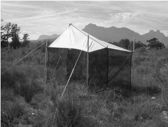
Fig. 4.20 Malaise trap. This catches insects both actively, by attracting certain insects, especially flies, by its dark form, and passively, by some insects inadvertently flying into it. On hitting the black gauze, the insects fly upwards and are guided by the tent cover into a bottle at the highest point containing a preservative, such as 70% ethanol (Courtesy James Pryke).
