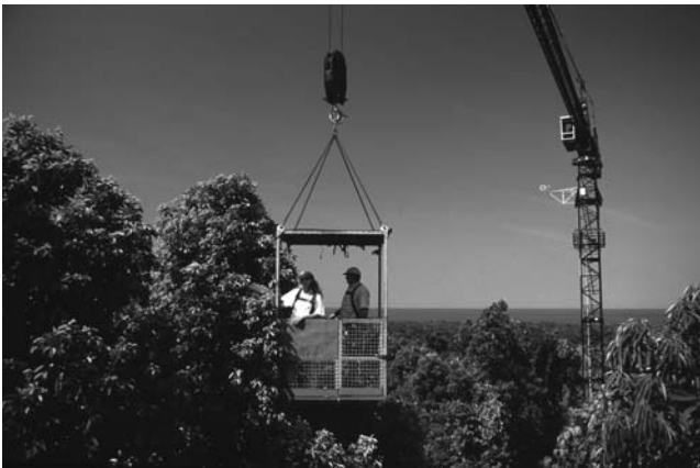
Fig. 4.2 A gondola suspended from the canopy research crane erected in the Queensland rainforest, Australia (Courtesy Nigel Stork).
