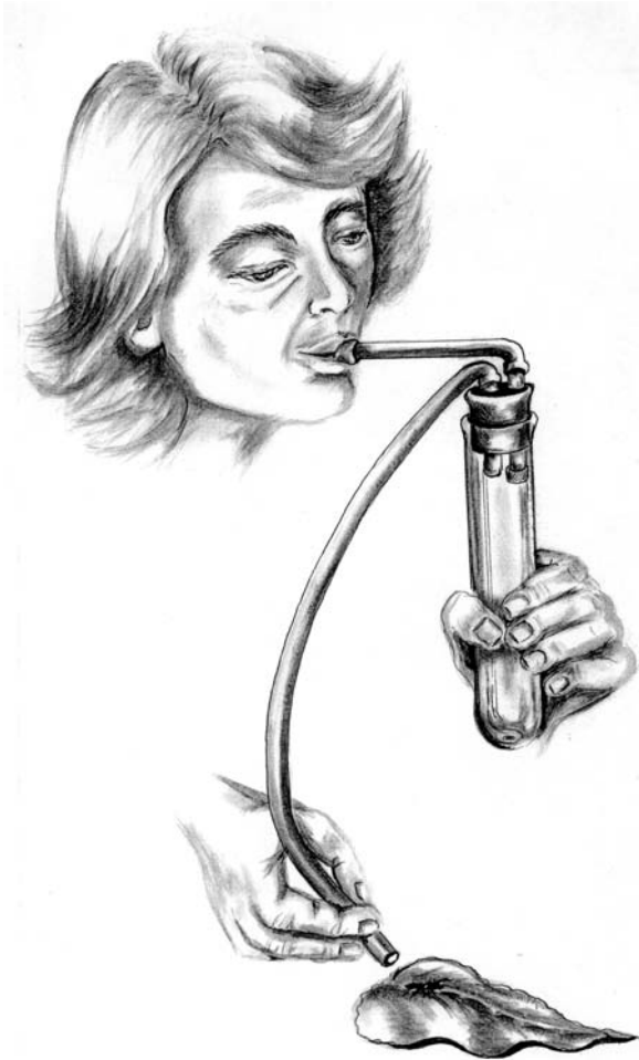
Fig. 4.6 Pooter (also called an aspirator) used for sucking up small insects from beating trays or directly from substrates.
