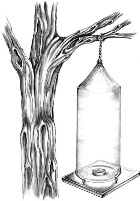
Fig. 4.23 Baited trap. This has a landing platform in the centre of which is placed a bait, such as rotting fruit. The trap consists of a net cylinder above the bait. Insects that land on the platform and head for the bait then tend to go upwards, and are trapped in the net.
