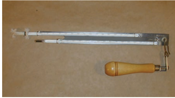
Figure 3.12 A sling type psychrometer (wet and dry bulb thermometer) used for determining relative humidity. The sling psychrometer is spun rapidly on its handle for approximately 1 minute before the reading is taken. Evaporative cooling of the moistened cotton wick of the wet bulb thermometer produces a lower than ambient temperature reading. The difference in temperatures is then utilized to determine the relative humidity. (Photo courtesy of Dr. Jason H. Byrd.)
