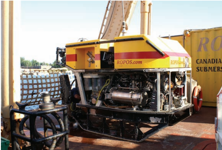
Figure 5.6 The Remote Operated Platform for Ocean Science (ROPOS), used to place equipment, the camera tripod, and the carcass in the Saanich Inlet, British Columbia, for underwater study. (Photo courtesy of Dr. Gail Anderson.)
