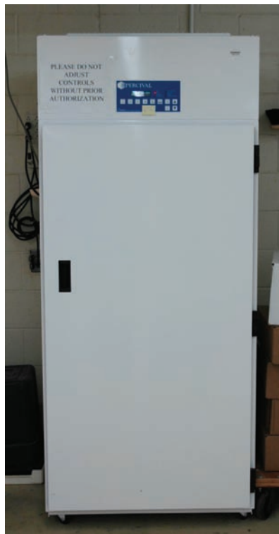
Figure 4.1 Typical reach-in type environmental chamber that controls light, temperature, and humidity for large numbers of insects. Such chambers are used for casework or research on insect growth and development. (Photo courtesy of Dr. Jason H. Byrd.)
