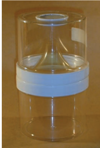
Figure 4.14 A commercially available rearing container that can be used for rearing terrestrial flying and some aquatic flying insects. The container is fitted with a cone that directs newly emerged adults into the vented top portion, where they are held until the container is emptied. (Photo courtesy of Dr. Jason H. Byrd.)
