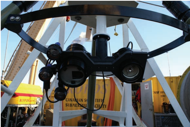
Figure 5.7 Camera, housing, and lighting array used to observe underwater carcass in Saanich Inlet in VENUS project. Camera and tripod deployed at a depth of 94 m in Saanich Inlet by ROPOS (Figure 5.6). (Photo courtesy of Dr. Gail Anderson.)
