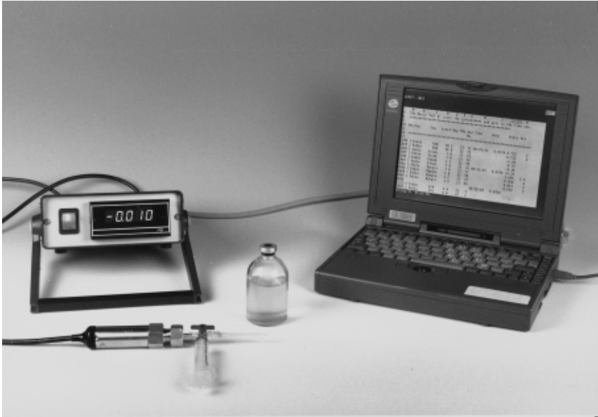
Fig. 10.2. The pressure transducer, complete with serum bottle, connectors and computer, as used for the manual transducer technique.
