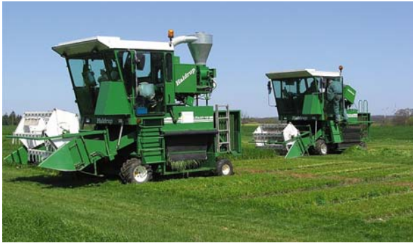
Fig. 3 Forage plot harvesters equipped with a sampling device and a Near-Infrared Reflectance Spectrometer for 'online' dry matter and quality determination (Photo U. Feuerstein)
