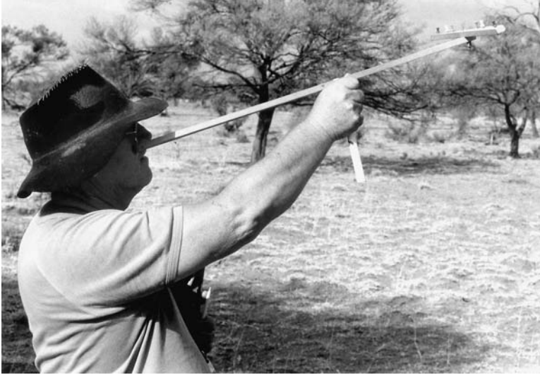
Fig. 10.4. The Bitterlich gauge for estimating total crown cover of trees and shrubs. Various pin spacings on the cross-bar provide gauge angles appropriate to different densities of trees and shrubs.
