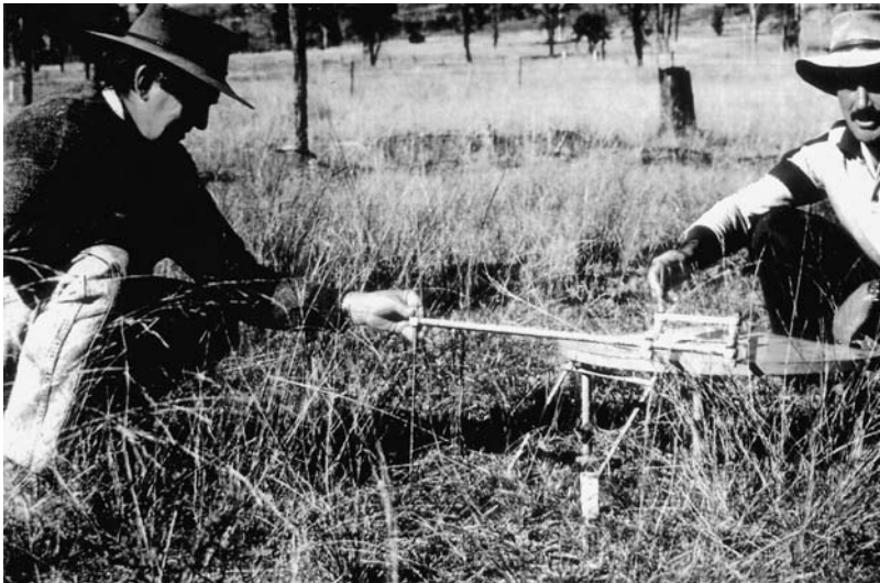
Fig. 6.2. A pantograph being used to measure basal cover of grasses in a sub-tropical native grassland.
