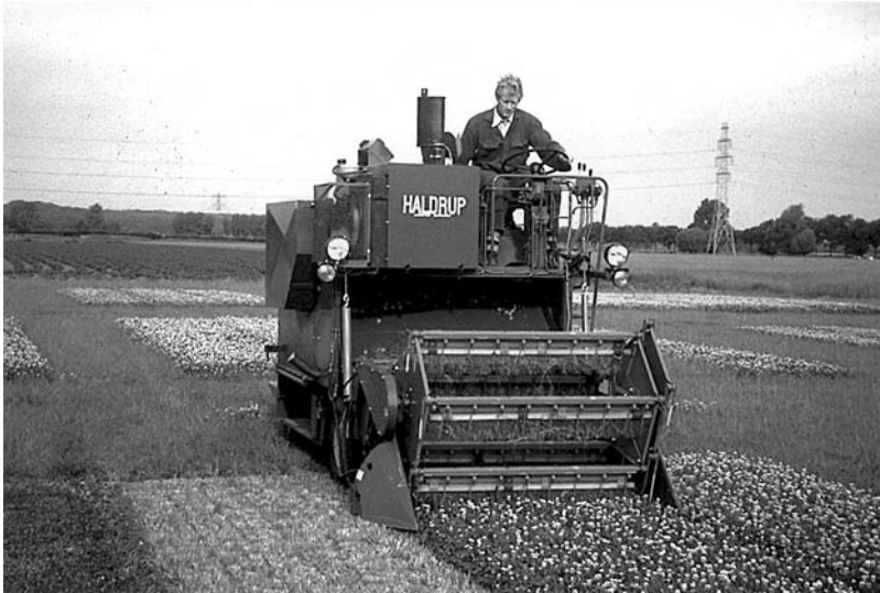
Fig. 7.1. Self-propelled weight recording plot harvester.
