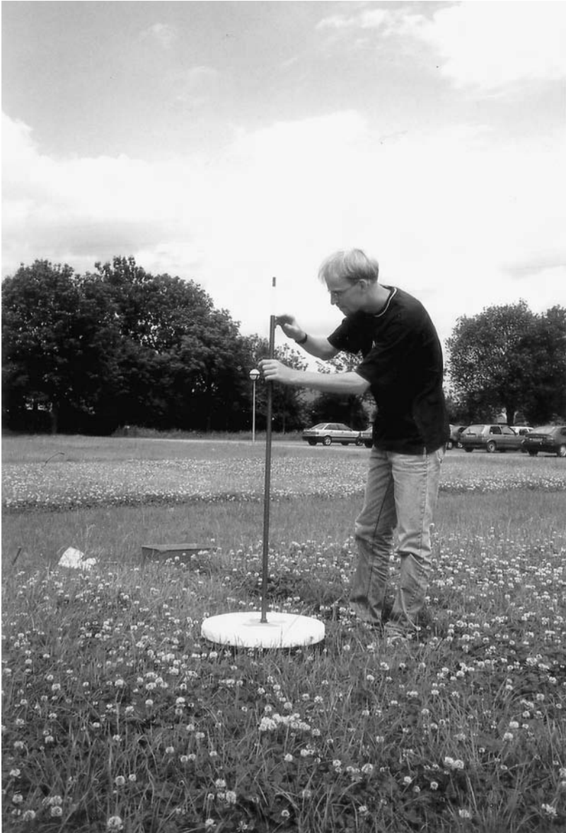
Fig. 7.2. Sward height meter consisting of a plastic disc that can move along a central rod with a height indicator at top.
