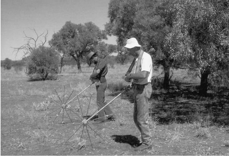
Fig. 10.3. Wheelpoint apparatus, for estimating aerial or basal cover of the understorey, as a one-person operation. The apparatus can be strapped to a belt, leaving the operator with hands free to record data on a small data logger slung from the neck in a comfortable position.
