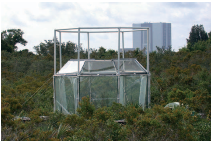
FIGURE 2 Open-topped chamber at Kennedy Space Center, Florida used to elevate atmosphere CO 2 .
