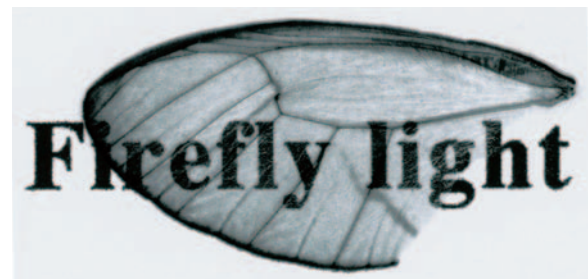
FIGURE 8 Effects of an antiglare coating. Even though the wing of this clearwing moth is somewhat wrinkled and parts of it would therefore be expected to reflect light, its matte surface (Fig. 9) allows the text to be read through it with minimal loss.
