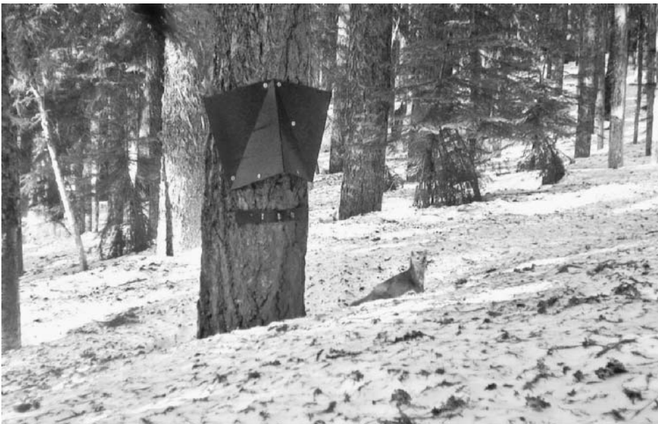
A pine marten visits a tree cubby device designed to snag a hair sample when the marten climbs inside to get the bait. (Western Transportation Institute)
