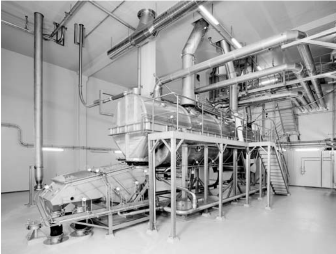
Fig. 3.17 Vibro-Fluidizer and sieve with side-mounted cleaning-in-place (CIP) nozzles. Data by permission of A.J. Partridge (personal communication) and GEA Process Engineering (Niro A/S), Gladsaxevej 305, Soeborg, Denmark.
