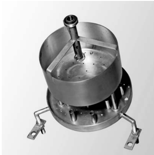
Fig. 3.1 A general view of the distribution plate in an evaporator showing the flow distribution system. Reproduced with the permission of NIZO Food Research B.V., Ede, The Netherlands.
