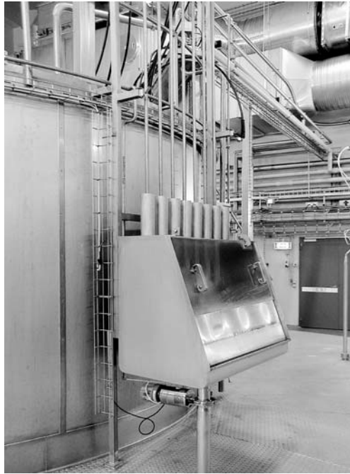
Fig. 3.15 High-pressure atomiser nozzles ready for cleaning-in-place (CIP) nozzles, and all nozzle lances and nozzle heads are placed in a special stand for cleaning. Data by permission of A.J. Partridge (personal communication) and GEA Process Engineering (Niro A/S), Gladsaxevej 305, Soeborg, Denmark.
