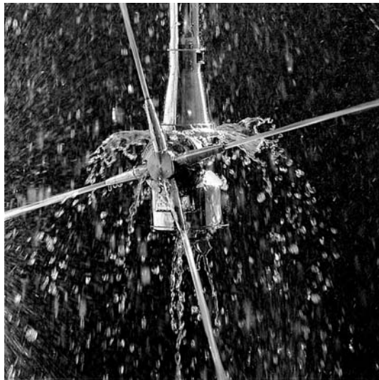
Fig. 3.19 Jet liquid nozzle for cleaning of the drying chamber surface. Data by permission of A.J. Partridge (personal communication) and GEA Process Engineering (Niro A/S), Gladsaxevej 305, Soeborg, Denmark.
