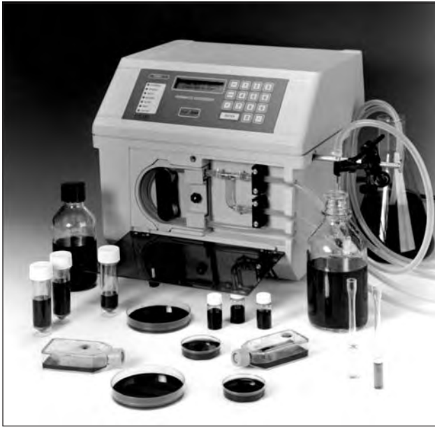
Fig. 5.9. Automatic Dispenser. The Perimatic Premier, suitable for repetitive dispensing and dilution in the 1- to 1000-mL range. If the device is used for sterile operations, only the delivery tube needs to be autoclaved.
