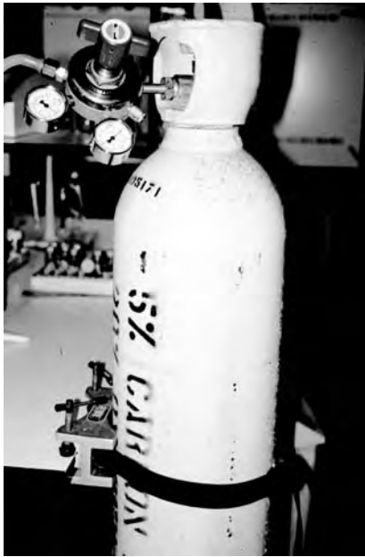
Fig. 7.3. Cylinder Clamp. Clamps onto edge of bench or rigid shelf and secures gas cylinder with fabric strap. Fits different sizes of cylinder and can be moved from one position to another if necessary; available from most laboratory suppliers.
