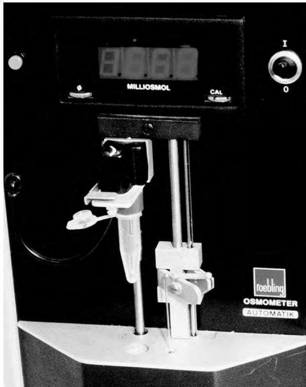
Fig. 9.1. Osmometer. Roebling osmometer (Camlab) showing front panel, sample tube, and sample port. This model accepts samples of 50 \mu L.
