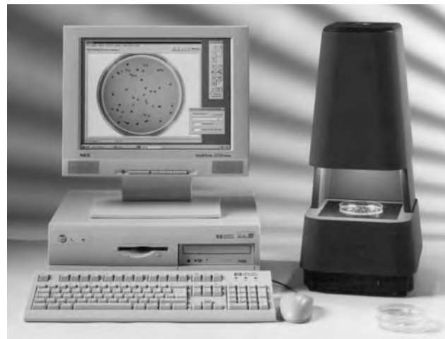
Fig. 21.12. Automatic Colony Counter. Automatic counter for colonies in plating efficiency and survival assays. (Perceptive Biosystems).
