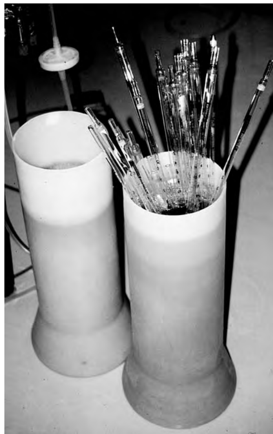
Fig. 7.1. Overfilled Pipette Cylinder. Pipettes protruding from a pipette cylinder as a result of attempted insertion of pipettes after the cylinder is full; those protruding from the cylinder will not soak properly or be disinfected and are prone to breakage (if glass) when other pipettes are added.
