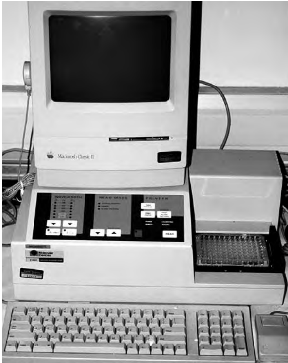
Fig. 5.12. Plate Reader. Densitometer for measuring absorbance of each well; some models also measure fluorescence. (Courtesy of Centre for Oncology and Applied Pharmacology, Glasgow University.)
