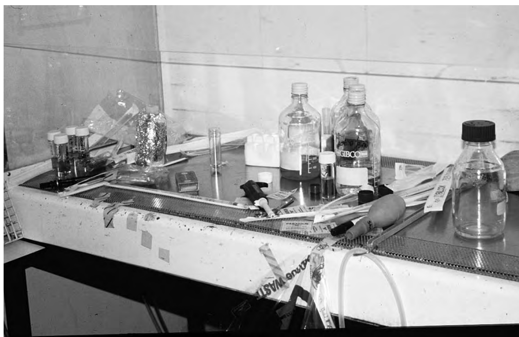
Fig. 6.3. Badly Arranged Work Area. Laminar-flow hood being used incorrectly. The hood is too full, and many items encroach on the air intake at the front, destroying the laminar airflow and compromising both containment and sterility.
