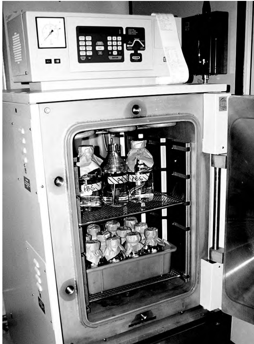
Fig. 5.19. Freestanding Autoclave. Medium-sized (300 L; 10 ft 3 ) laboratory autoclave with square chamber for maximum load. The recorder on the top console is connected to a probe in the bottle in the center of the load. (Courtesy of Beatson Institute).
