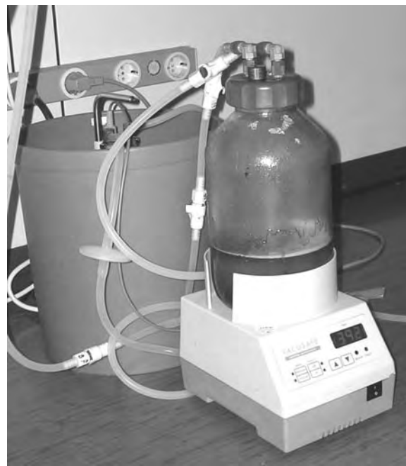
Fig. 5.3. Integra Vacuum Pump. Suction pump and receiver for removing fluids from flasks; available from Integra. (Courtesy of Norbert Fusenig, Deutsches Krebsforschungszentrum, Heidelberg).
