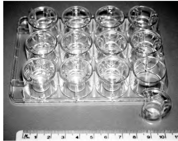
Fig. 25.8. Transwells. Filter well inserts in a twelve-well plate, with a filter well insert alongside. (Corning.)
