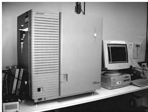
Fig. 16.10. DNA Sequencer. ABI 377 DNA sequencer using automated electrophoretic analysis on polyacrylamide gel to separate and quantify amplified STR sequences. (Photo courtesy of A. James, LGC Promochem).
