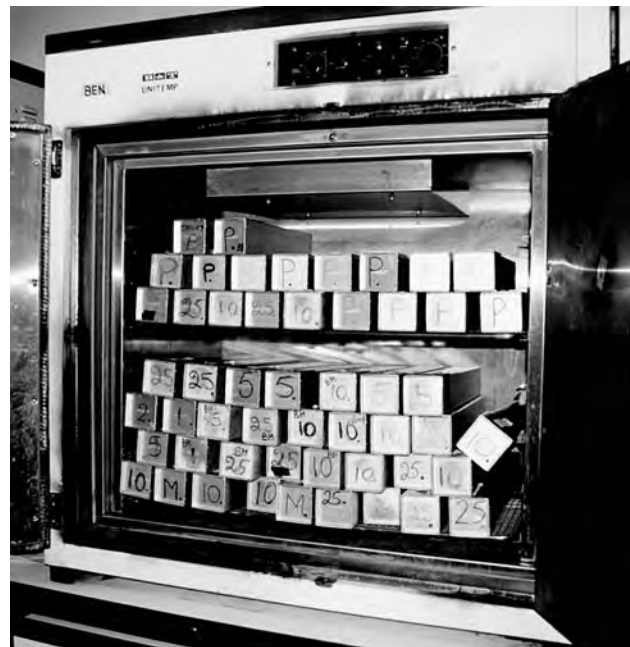
Fig. 11.7. Sterilizing Oven. Pipette cans are stacked with spaces between to allow circulation of hot air. Brown staining on front of oven shows evidence of volatile material from sterile-indicating tape.
