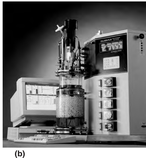
Fig. 26.15. Fixed-Bed Reactors. Cells grown on the surface of beads or macrocarriers are perfused with medium. The beads are usually glass and are settled in a dense bed resting on a perforated base at the bottom of the culture vessel, or, if of a lighter material, are restrained within a cage. Once the culture is established, the beads do not move, and medium percolates around them. (a) Hypothetical diagram. (b) Celligen reactor (Courtesy of New Brunswick Scientific).
