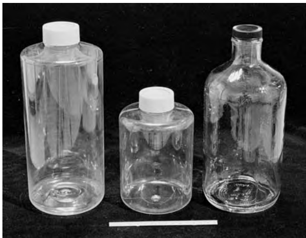
Fig. 26.13. Examples of Roller Culture Bottles. Center and left, disposable plastic (Falcon, Corning); right, glass.
