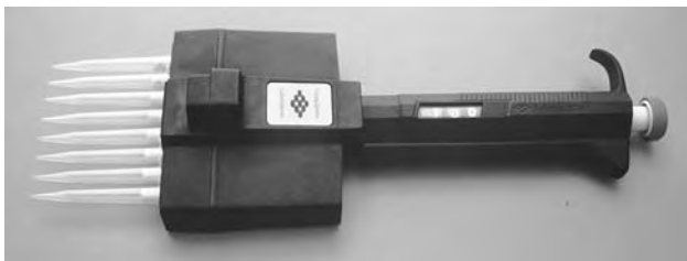
Fig. 5.10. Multipoint Pipettor. Pipettor with manifold to take 8 plastic tips. Also available for 4 and 12.
