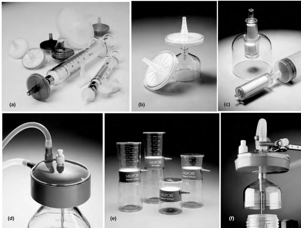
Fig. 11.12. Disposable Sterilizing Filters. (a) Millex 25-mm disk syringe filter. (b) In-line filter with bell. (c) Sterivex with and without bell. (d) Bottle-top filter. (e) Filter cup and storage vessels. (f) Large in-line filter with bell. (a,b,c,f) Positive pressure. (d,e) Negative pressure (see also Fig. 11.11). Photographs courtesy of Millipore (UK), Ltd.
