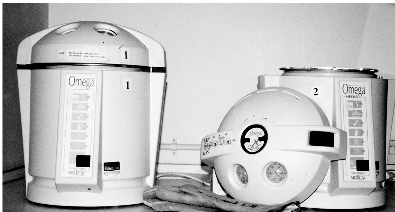
Fig. 5.18. Bench-Top Autoclave. Simple, top-loading autoclave from Prestige Medical; left with lid closed, right with lid removed for filling. (Courtesy of Beatson Institute.)
