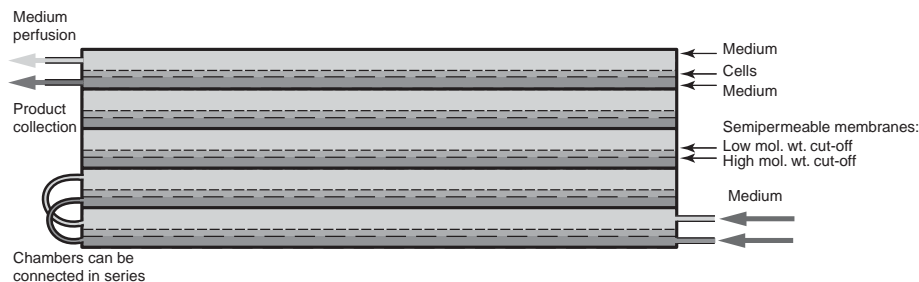
Fig. 26.7. Membroferm. Membroferm three-compartment membrane reactor [Klement et al., 1987]. A lamellate structure of semipermeable membranes, based on a triple unit wherein cells within a double membrane are fed from an upper compartment via a membrane with a low-molecular-weight cutoff. The cells secrete product into the lower compartment via a membrane that is microporous with a high-molecular-weight cutoff. Each base unit of three elements can be connected to create a perfusion system with the medium layer and product layers separate or combined.
