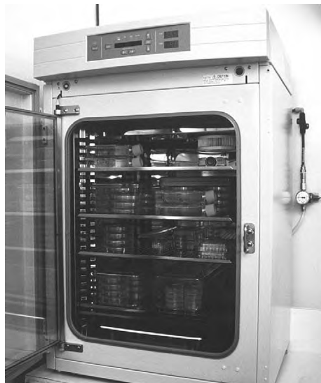
Fig. 5.15. CO 2 Incubator. CO 2 incubator (Forma) with door open showing flasks, multiwell plates and boxed Petri dishes. ( see also Fig. 5.16).
