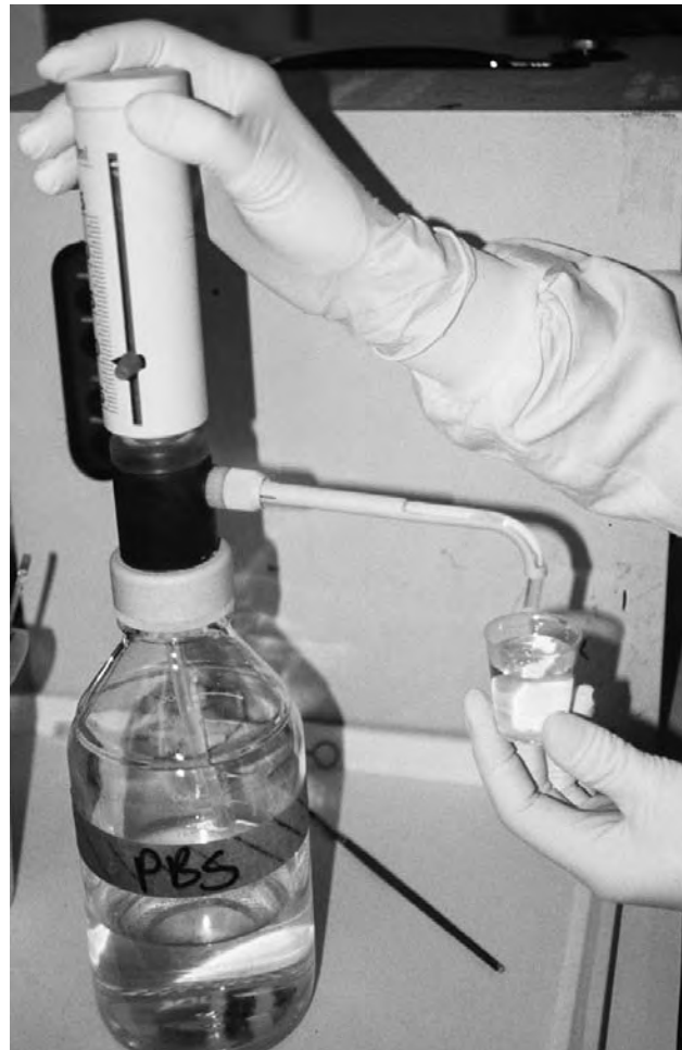
Fig. 5.20. Bottle-Top Dispenser. Spring-loaded piston connected to a two-way valve, alternately drawing a preset volume from the reservoir and dispensing through a side arm. The device is useful for repetitive dispensing of nonsterile solutions such as PBSA for cell counting. Some models can be autoclaved for sterile use.
