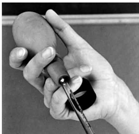
Fig. 6.6. Holding Cap and Bulb. Cap may be unscrewed and held in the crook of the little finger of the hand holding the bulb or pipetting aid.
