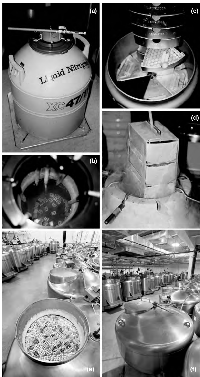
Fig. 20.6. Liquid Nitrogen Freezers. (a) Narrow-necked freezer with storage on canes in canisters. (b) Interior of the narrow-necked freezer, looking down on canes in canister, positioned in center as it would be for withdrawal. Normal storage position is under shoulder of freezer, just visible top right. (c) Wide-necked freezer with storage in triangular drawers. (d) Narrow-necked freezer with storage in square drawers ( see also Fig. 20.7). (e) High-capacity freezer with offset access port open, revealing canes in canisters. (f) High-capacity freezers in a cell bank. Nearest freezer shows connections for monitoring and automatic filling. (e & f, photos courtesy of ATCC.)
