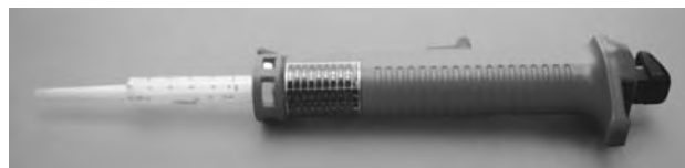
Fig. 5.8. Repette. Stepping dispenser operated by incremental movement of piston in syringe, activated by thumb button (Jencons).
