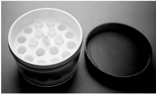
Fig. 20.4. Nalge Nunc Cooler. Plastic holder with fluid-filled base. The specific heat of the coolant in the base insulates the container and gives a cooling rate of \sim 1^\circ\text{C}/\text{min} in the ampoules.
