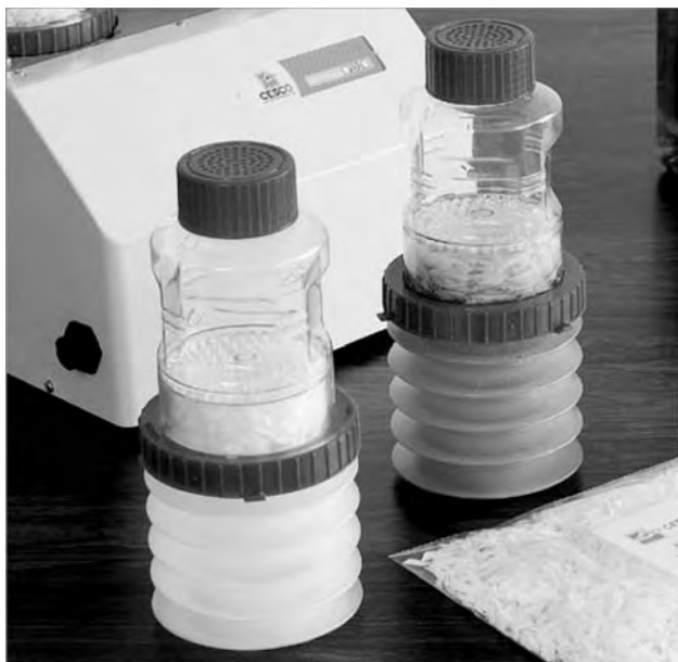
Fig. 26.5. BelloCell Aerator Culture. Cells are grown on matrix material that is alternately submerged in medium and exposed for gas exchange by pumping of the bellows compartment.
