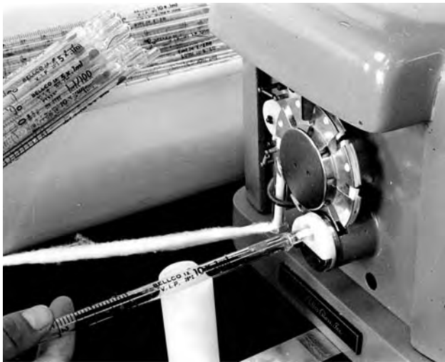
Fig. 11.6. Semiautomatic Pipette Plunger (Bellco). A thick strand of cotton is fed through a selected loading aperture, and a section is cut off when the appropriate length is inserted in the end of the pipette. Different thicknesses of cotton are required for different sizes of pipette.
