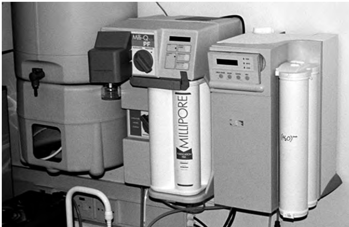
Fig. 5.17. Water Purifier. Tap water first passes through a reverse-osmosis unit on the right and then goes to the storage tank on the left. It then passes through carbon filtration and deionization (center unit) before being collected via a micropore filter (Millipore Milli-Q). (Courtesy of Beatson Institute).
