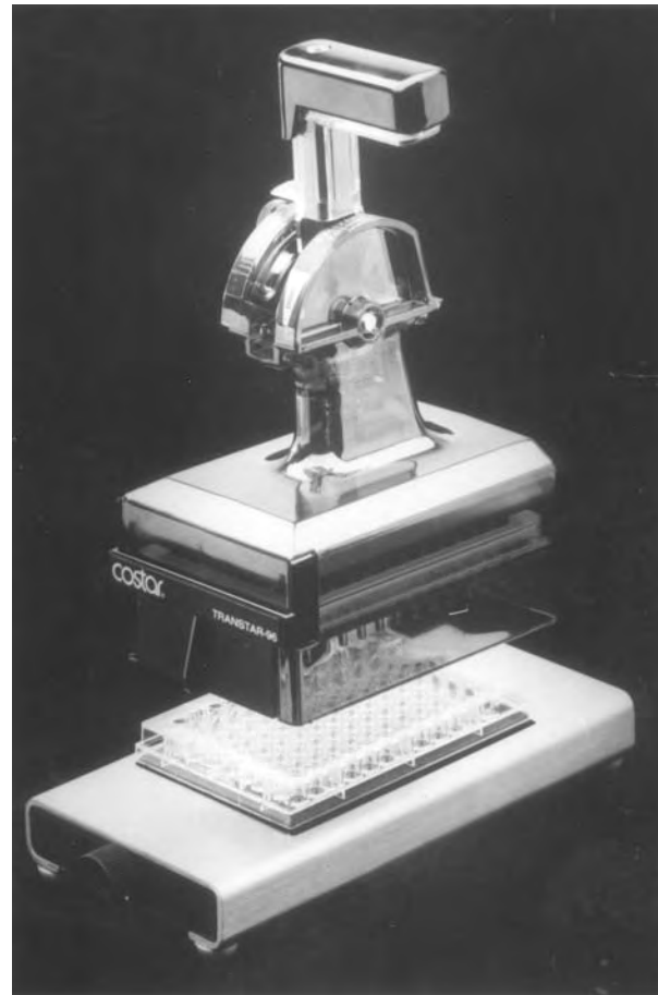
Fig. 5.13. Transfer Device. Transtar (Corning) for seeding, transferring medium, replica plating, and other similar manipulations with microtiter plates, enabling simultaneous handling of all 96 wells. (Reproduced by permission of Corning).
