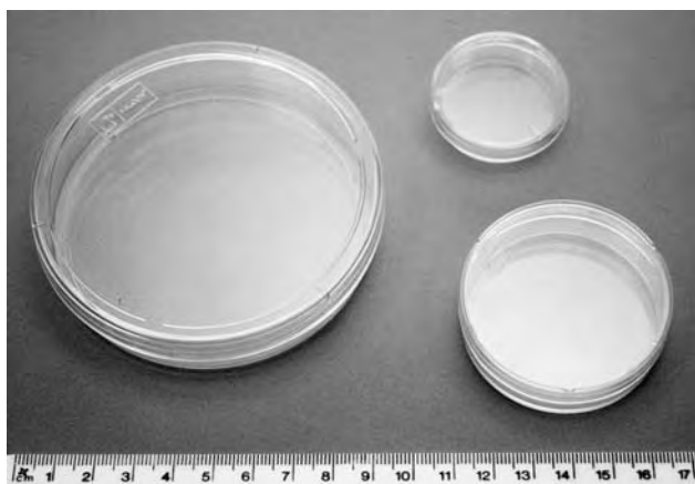
Fig. 8.3. Petri Dishes. Illustrated are dishes of 3.5-cm, 5-cm, and 9-cm diameter. Square Petri dishes are also available, with dimensions 9 × 9 cm. A grid pattern can be provided to help in scanning the dish—for example, in counting colonies—but can interfere with automatic colony counting.
