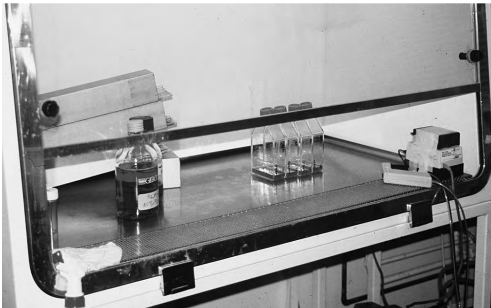
Fig. 6.2. Suggested Layout of Work Area. Laminar-flow hood laid out correctly. Positions may be reversed for left-handed workers.
