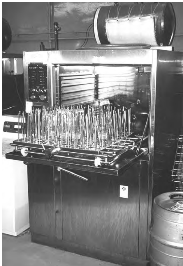
Fig. 5.21. Glassware Washing Machine. Glassware is placed on individual jets, which ensures thorough washing and rinsing (Betterbuilt). (Courtesy of Beatson Institute).
