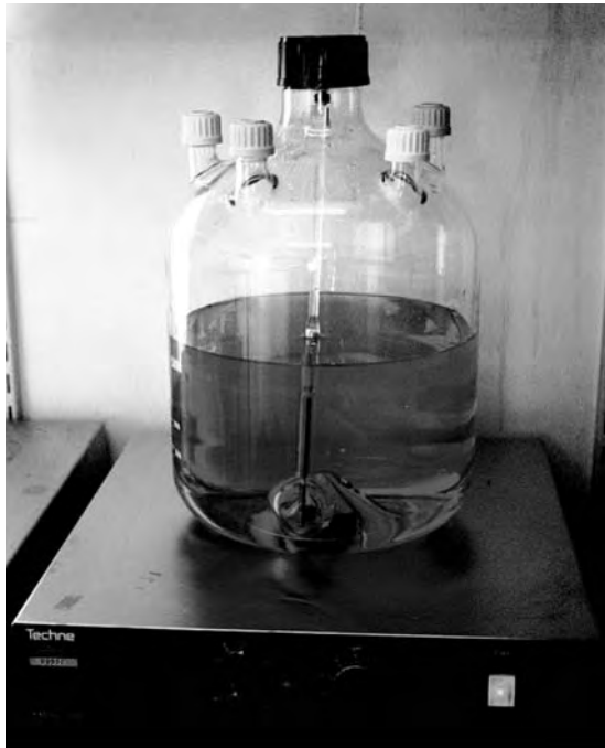
Fig. 26.1. Large Stirrer Flask. Techne 5-L stirrer flask on a magnetic stirrer. Note the offset pendulum that makes an excursion in the annular depression in the base of the flask. The side arms are for sampling or perfusion with CO 2 in air, which would be required with this volume of medium (see Figure 26.2).
