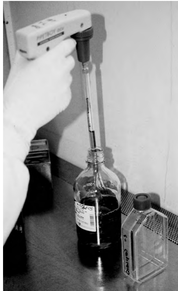
Fig. 5.5. Pipetting Aid. Motorized pipetting device for use with conventional graduated pipettes.
