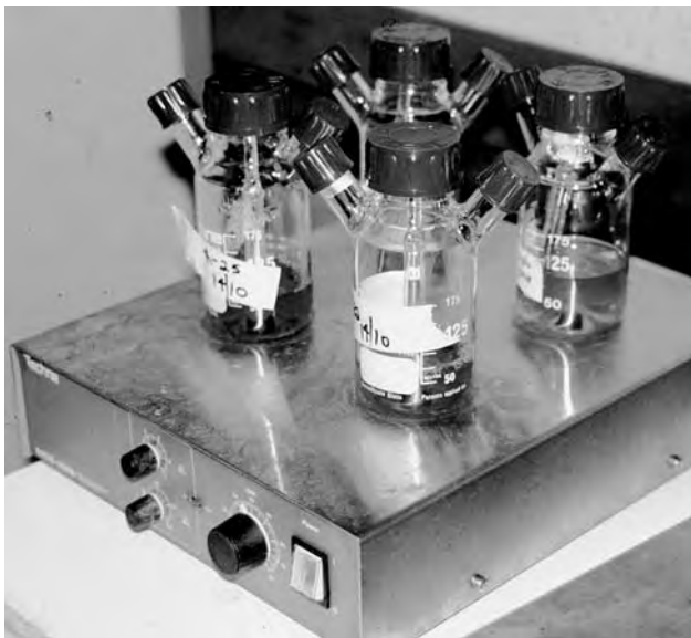
Fig. 8.6. Small Stirrer Flasks. Four small stirrer flasks (Techne), 250-mL capacity, with 50–100 mL medium, on four-place stirrer rack (Techne). Larger flasks, up to 10 L, are available ( see also Figs. 13.5, 26.1, 26.2).
