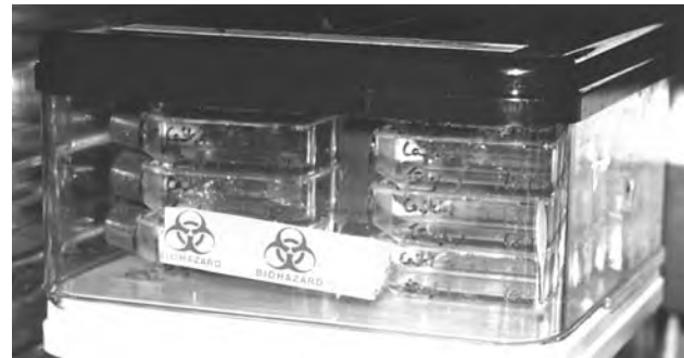
Fig. 6.10. Boxed Dishes. A transparent box, such as a sandwich box or cake box, helps to protect unsealed dishes and plates, and flasks with slacked caps, from contamination in a humid incubator. This type of container should also be used for materials that may be biohazardous, to help contain spillage in the event of an accident.
