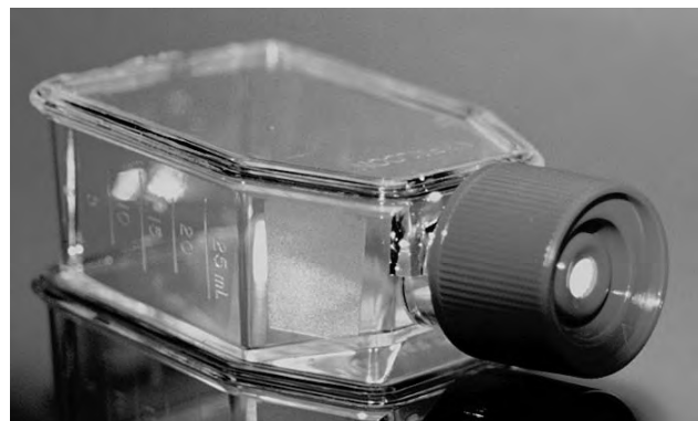
Fig. 8.8. Venting Flasks. Gas-permeable cap on 10-cm 2 flask (Falcon, B-D Biosciences).
