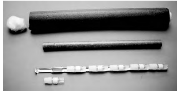
Fig. 20.2. Ampoules on Cane. Plastic ampoules are clipped onto an aluminum cane (bottom), enclosed in a cardboard tube (middle), and placed inside an insulating foam tube (top). The insulating tube is plugged at either end with cotton or another suitable insulating material.
