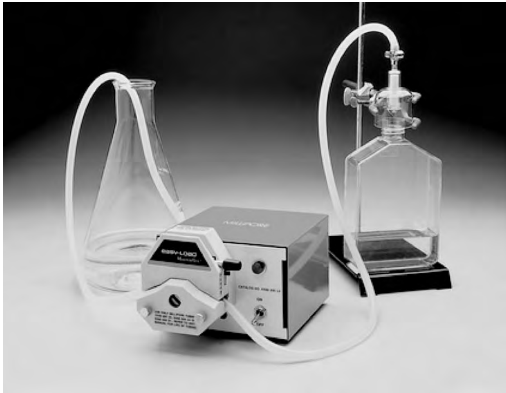
Fig. 11.14. Peristaltic Pump Filtration. Sterile filtration with peristaltic pump between nonsterile reservoir and sterilizing filter (Millipak, Millipore; courtesy of Millipore [U.K.], Ltd).
