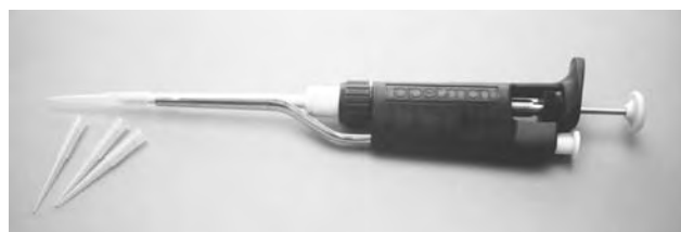
Fig. 5.6. Pipettor. Variable-volume pipetting device. Also available in fixed volume. The pipettor is not itself sterilized but is used with sterilized plastic tips.
