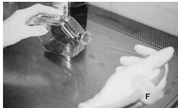
Fig. 6.11. Gassing a Flask. A pipette is inserted into the supply line from the CO 2 source, and the 5% CO 2 is used to flush the air out of the flask without bubbling through the medium. The letter F indicates a micropore filter inserted in the CO 2 line.
