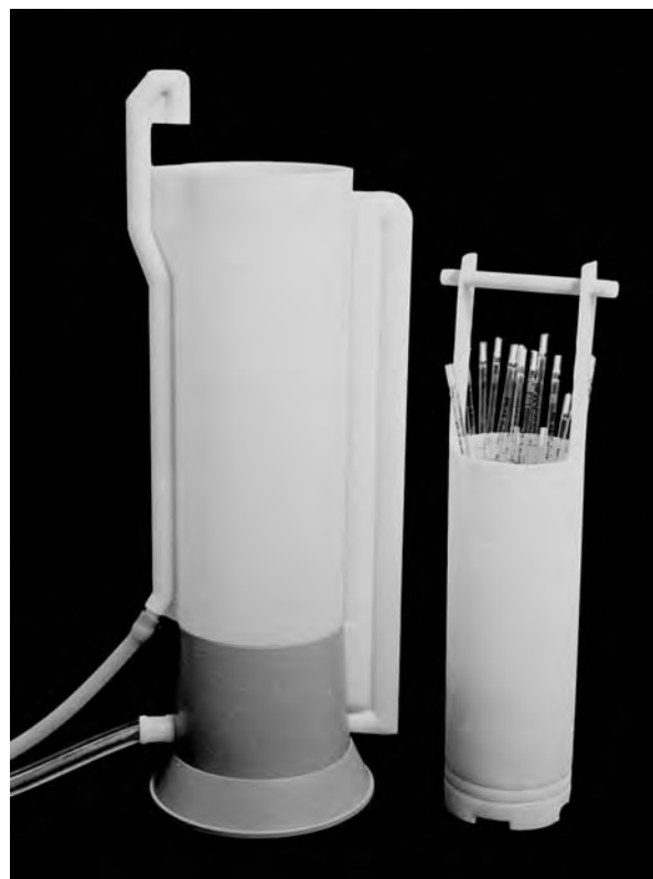
Fig. 11.4. Siphon Pipette Washer. Connected to main water supply. A slow fill establishes a siphoning action and drains the main chamber, which then refills. This process is repeated many times over 4–6 h. The pipettes shown here are as collected from use. Before the pipette basket is placed in the washer, the plugs are blown out and the pipettes inverted, as in Fig. 11.5.
