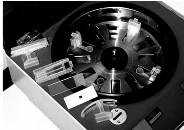
Fig. 16.4. Cytocentrifuge. View of interior of centrifuge showing rotor and polypropylene slide carriers in place with one carrier disassembled on left-hand side (Sakura Finetek).
