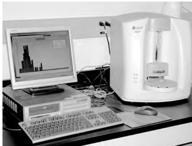
Fig. 21.5. Beckman Coulter Vi-CELL Electronic Cell Counter. An undiluted cell suspension is placed in a cup in the sample holder, sampled by the counter (right), mixed with Trypan Blue, and analyzed in a flow cell. The output appears on the display (left) as a graphic of cell size distribution or a microscope view of the cells with live cells circled in green and dead cells circled in red. (Courtesy of ATCC).
