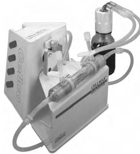
Fig. 8.11. Hollow Fiber Culture. A bundle of hollow fibers of permeable plastic is enclosed in a transparent plastic outer chamber and is accessible via either of the two side arms for seeding cells. During culture, the chamber is perfused down the center of the hollow fibers through connections attached to either end of the chamber (CellMax, Spectrum Labs; see also Fig. 26.6).
