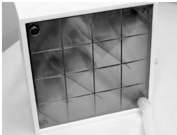
Fig. 26.10. Corning CellCube. Multisurface cell propagator with 6500-cm 2 available growth surface. (Courtesy of ATCC.)
