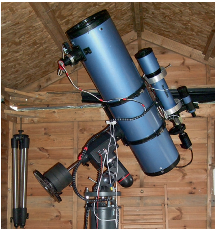
Fig. 9.2. 80 mm f/7 refractor piggybacked onto a 250 mm f/5 Newtonian reflector.
