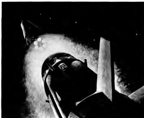
Top left, Saturn I SA-4 rises from the launch pad on 28 March 1963. The last of the Block I vehicles, it has no aerodynamic fins as does SA-5, which sits on the pad at top, right. At left is an artist's conception of S-IV stage separation in space, with the six RL-10 engines kicking the payload into orbit.
