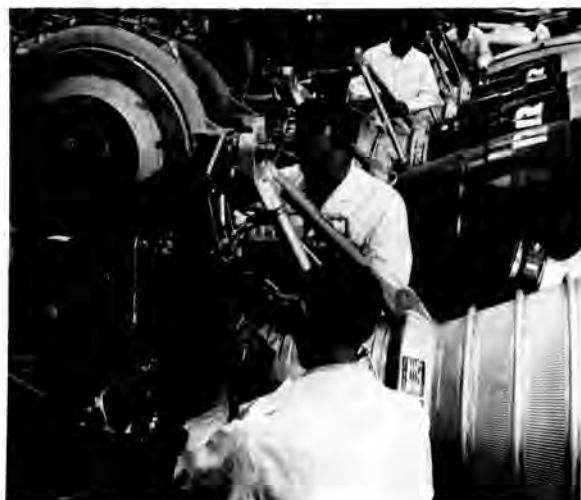
At left is shown a 1963 test firing of an H-1 engine on a Rocketdyne test stand. At right are H-1 engines in Rocketdyne's assembly line at Canoga Park, California.
