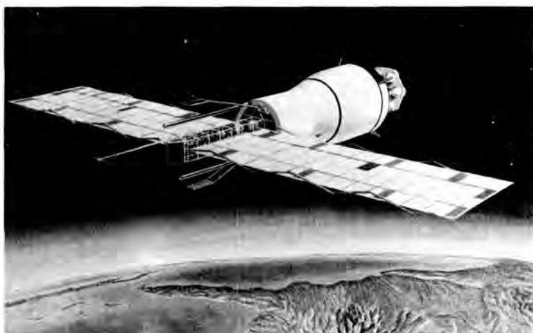
Above, a Fairchild technician checks out the extended Pegasus meteoroid detection surface in March 1964. At right is an artist's conception of Pegasus in orbit with meteoroid detector extended.
