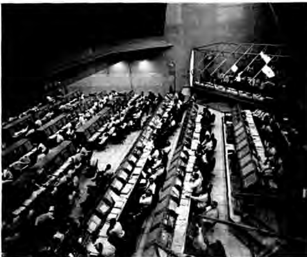
Computers and their end product devised for Saturn V—automatic checkout of flight hardware—were much in evidence at the Kennedy Space Center. This view of the control center, with row on row of computer consoles, is only one portion of the system.
