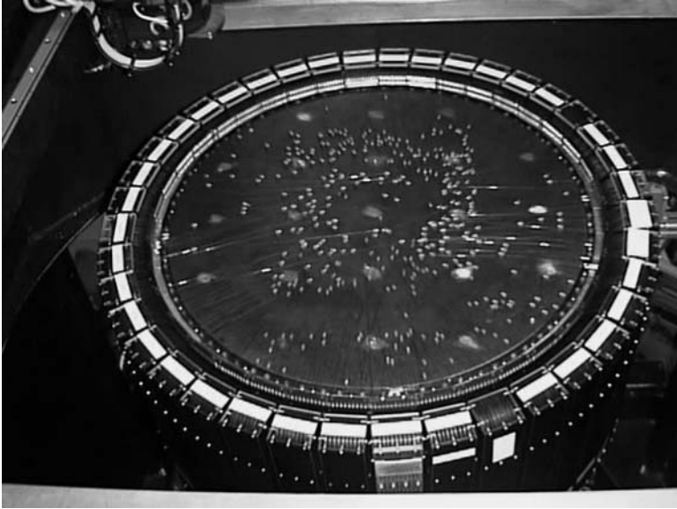
Fig. 4.10 Fiber-feed assembly for the fiber-fed multi-object spectrograph at the AAO 3.9-m telescope. This instrument was used for the 2dF Galaxy Redshift Survey ([106]). The assembly consists of 400 fiber ends on top of a metal plate in the focal plane of the telescope. Before each exposure the fiber ends are positioned at the coordinates of the spectroscopic targets by computer-controlled robot. During the exposure the feeds are magnetically attached to the focal-plane plate. (Photo and copyright: Anglo-Australian Observatory)
