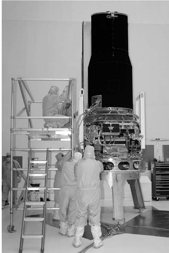
Fig. 4.2 The Spitzer infrared space observatory during the preparation for launch at NASA. The image shows the cooled 85-cm telescope on top of the instrument assembly. In space the telescope is shielded from the solar radiation by the solar panels visible behind the telescope tube. (Photo National Aeronautics and Space Administration)
