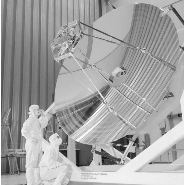
Fig. 12.6 The 3.5-m telescope of the HERSCHEL far-infrared space observatory during laboratory inspection at ESA. (Photo European Space Agency)
