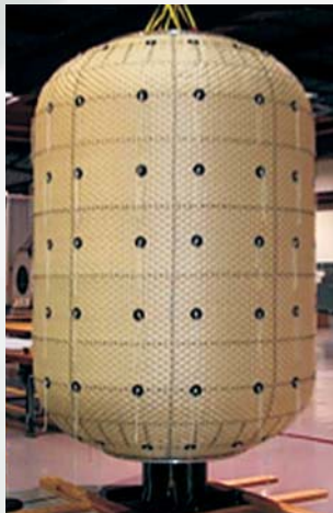
Below: A 2.24-metre diameter demonstration restraint layer being prepared for hydrostatic testing (top) at Johnson Space Center in November 2005. The fact that the restraint layer failed only at a pressure of 197 psi (13.85 kg/cm 2 ) demonstrated a factor of safety exceeding 4.0 (bottom). Images courtesy NASA/Chris Johnson/Gary Spexarth.
