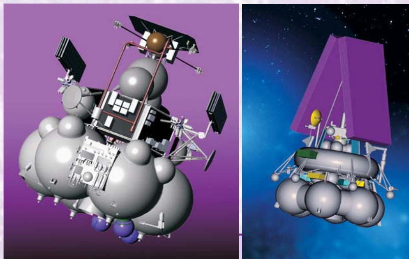
■ Above: Artist's schematics showing the Fobos Grunt spacecraft (comprising both the lander and the injection stage) prior to setting off for Mars (left), and the spacecraft during transit to Mars (right). Images courtesy Lavochkin Association.
