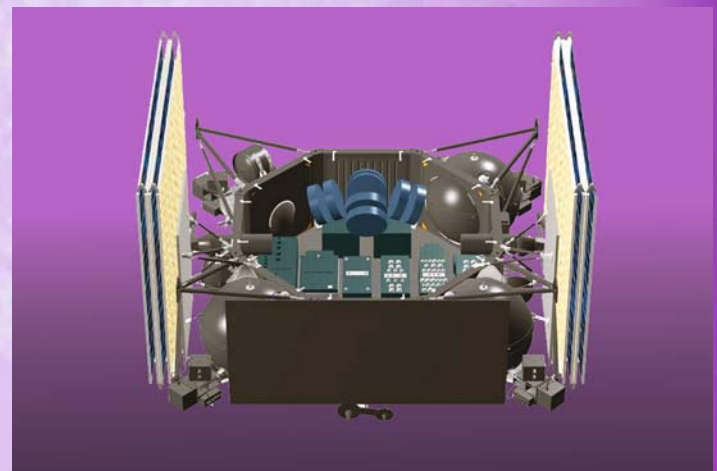
■ Below: Artist's schematic of the Navigator platform which has been used as a basis for the design of a range of new Russian space observatories, including the Spektr RG spacecraft. The Navigator platform is based on the Fobos Grunt platform designed for the mission to Mars' moon Phobos. Image courtesy IKI, Institute for Space Research, Moscow.
