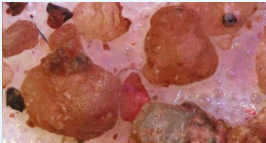
■ Above: An image of beach sand taken with the optical microscope in the laboratory. The larger particles are about half a millimeter across. The smallest are 10 microns. By analyzing the colours and shapes, quartz can be distinguished from biotite and feldspar. Image courtesy UA/LPL.
