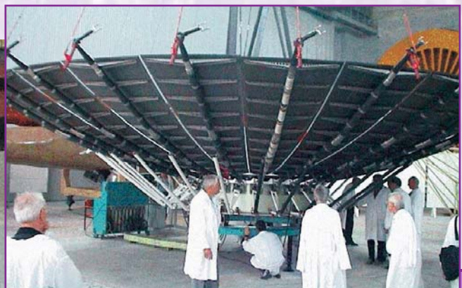
■ Above and left: Two views of the 10-m diameter main antenna of the Spektr R (Radioastron) space observatory being deployed during testing at the works of the Lavochkin Association during 2002. Images courtesy Lavochkin Association.
