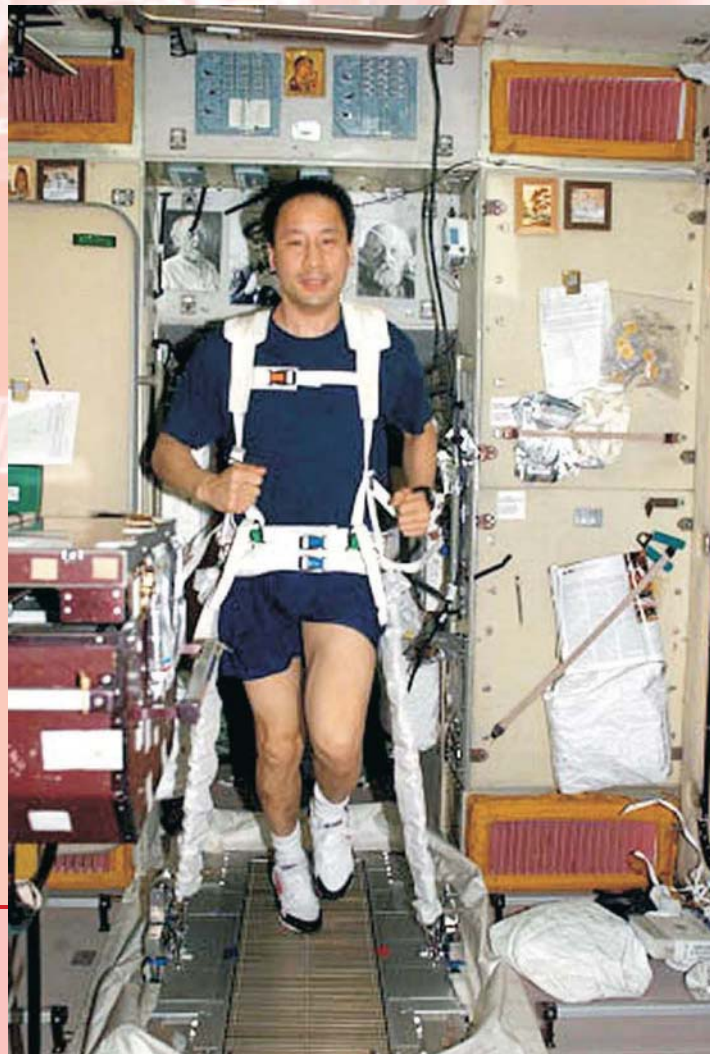
■ Right: NASA ISS Science Officer and Expedition 7 crew member Ed Lu exercising on the treadmill aboard ISS: the entire treadmill below his feet is floating in a big pit in the floor. Image courtesy NASA.
