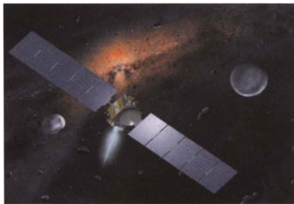
Dawn —The Dawn asteroid explorer shown with Vesta and Ceres against a background painting of a primordial solar nebula. Dawn will use ion engines during a nine-year mission that will enable it to enter orbit around both of these large primordial worlds. Its measurements will provide detailed insights into the nature of two very different bodies, and enable scientists to compare their characteristics with those of meteorites found on Earth. (UCLA/William Hartmann)
