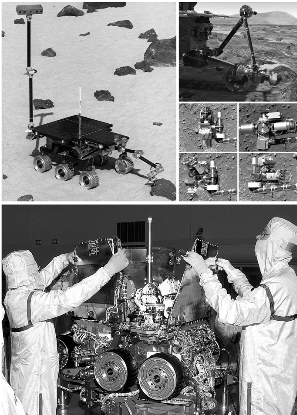
Technicians prepare one of the Mars Exploration Rover vehicles. The FIDO rover (top-left) was used to prepare for the mission. In its final form, the MER featured a robotic arm with a suite of instruments (top-right) to enable it to operate as a field geologist.
