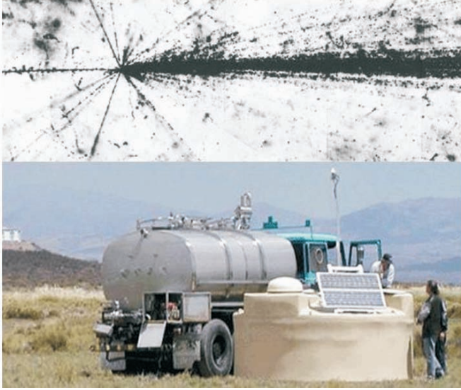
Figure 6.9: A collision between a high-energy cosmic ray particle and an atom in a photographic emulsion (viewed through a microscope). Below: filling of a water tank of the Auger observatory.
