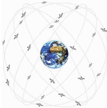
Figure 11.1: Orbits of GPS satellites. The satellites orbit the earth with a speed of 3.9 km/s. One revolution takes 12 h sidereal time, corresponding to 11 h 58 min earth time. This means that the same satellite reaches a certain position about 4 minutes earlier each day. The mean distance from the middle of the earth is 26560 km. The system consists of at least 24 satellites, the first one started in 1978. The European GALILEO will be operational in 2010, consisting of 30 satellites (27 working, 3 in reserve). http : //www.kowoma.de/en/gps/orbits.htm
